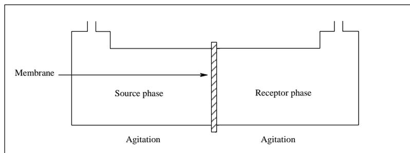
**Figure 2:** Scheme of the mounting used.
