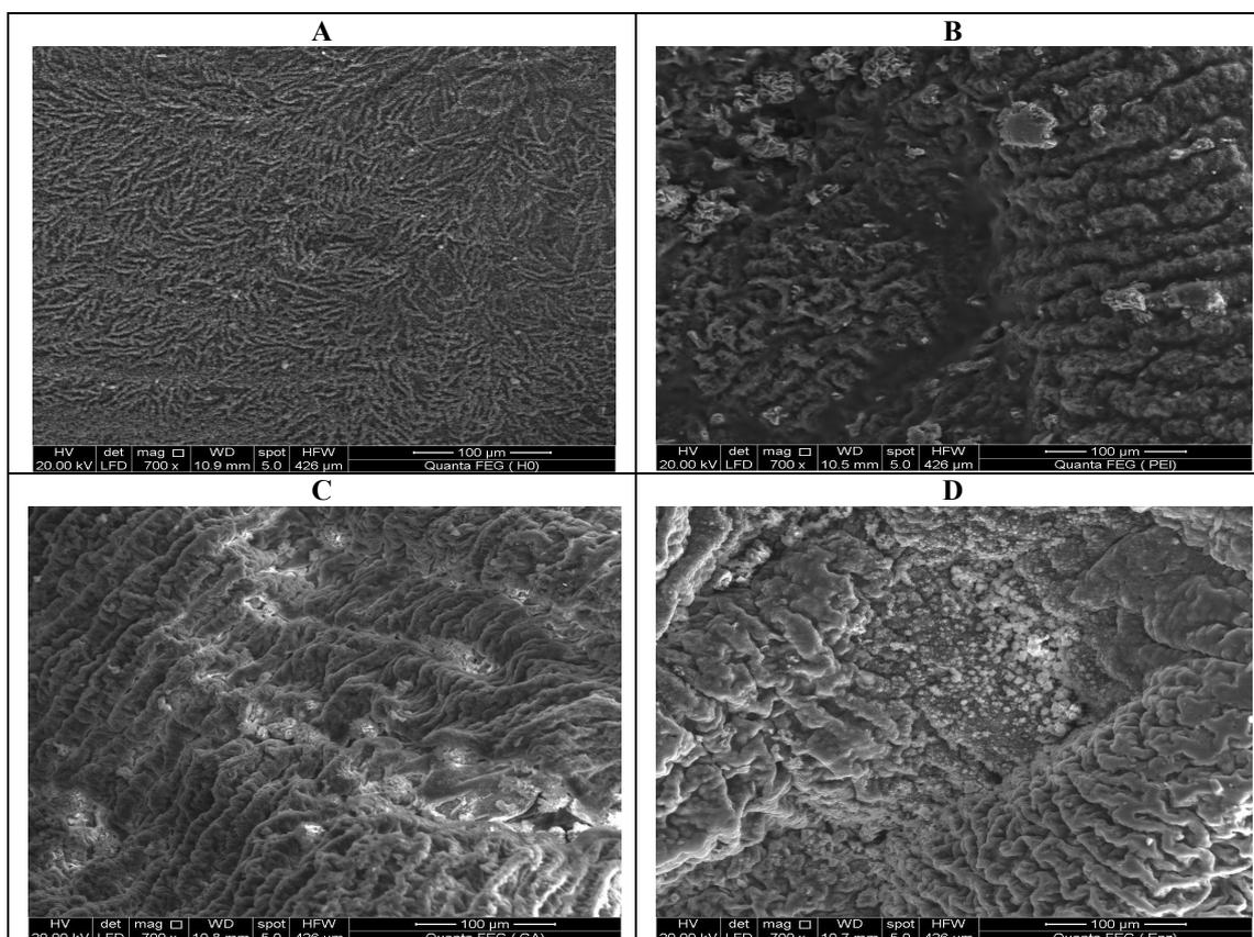
**Figure 7** SEM for surface of gel beads. Gel beads (A), aminated beads (B), activated beads (C) and immobilized one (D). At magnification of 700x
