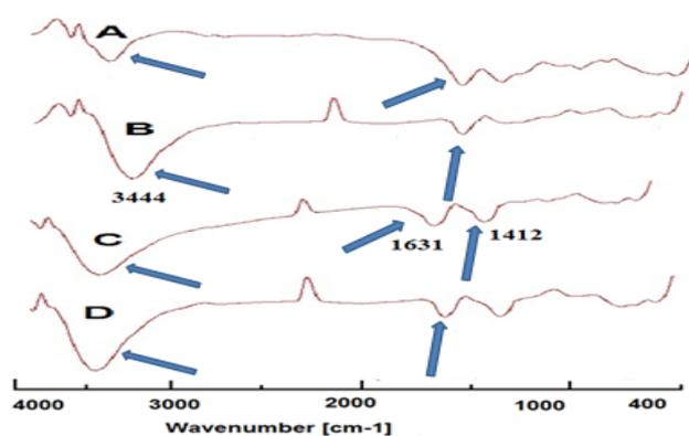
**Figure 5** FT-IR of H0. Gel beads (A), aminated beads (B), activated beads (C) and immobilized one (D).
