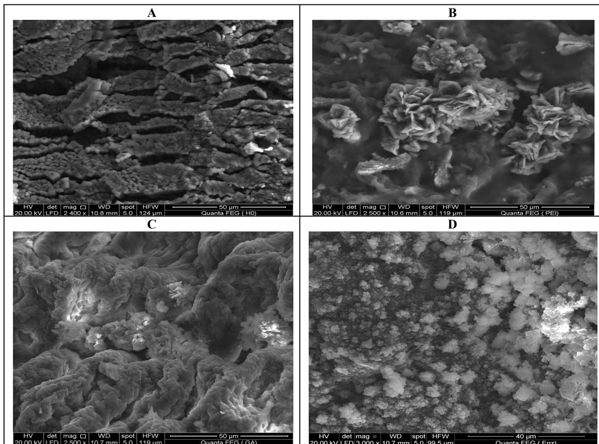
**Figure 8** SEM for surface of gel beads. Gel beads (A), aminated beads (B), activated beads (C) and immobilized one (D). At magnification of 2500x
