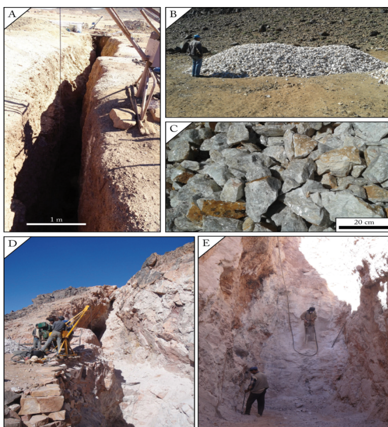
Figure 6: Exploitation of barite vein used in Drâa-Tafilalet region (A, d and E), appearance of barite after manual sorting, example of Tinejdad barite ore (B and C).
