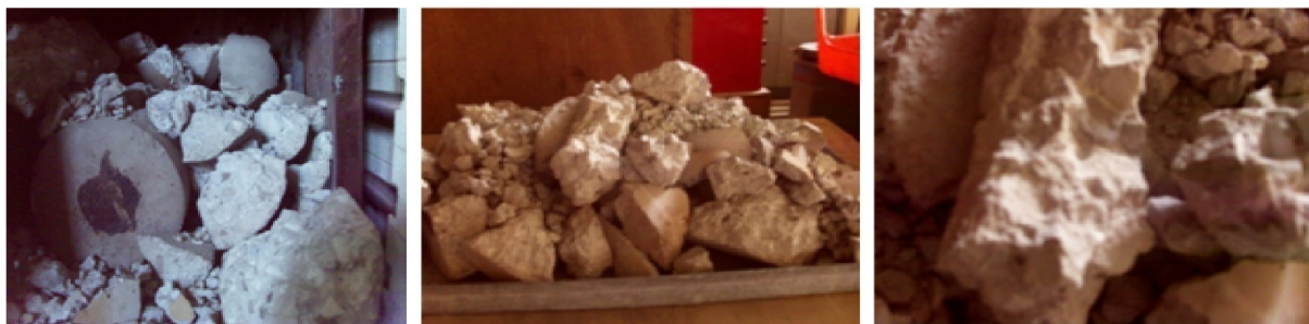
Figure 4: Explosive Burst of HPC2 at 544 ° C
