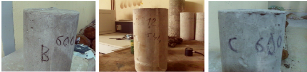
Figure 3: Appearance of significant cracks after 600 ° C (HPC)
