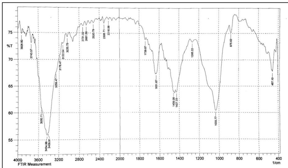
Figure 8. FT-IR spectra of punica granatum film adsorbed on amalgam surface after immersion and corrosion in saliva solution.
