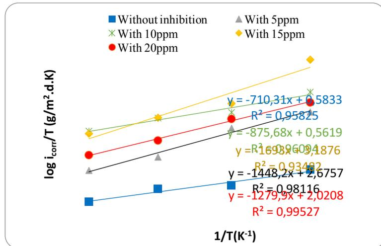
**Figure 4.** log CR/T Versus 1/T for the corrosion of amalgam in artificial saliva solution in absence and presence various (P.g.e) concentrations.
