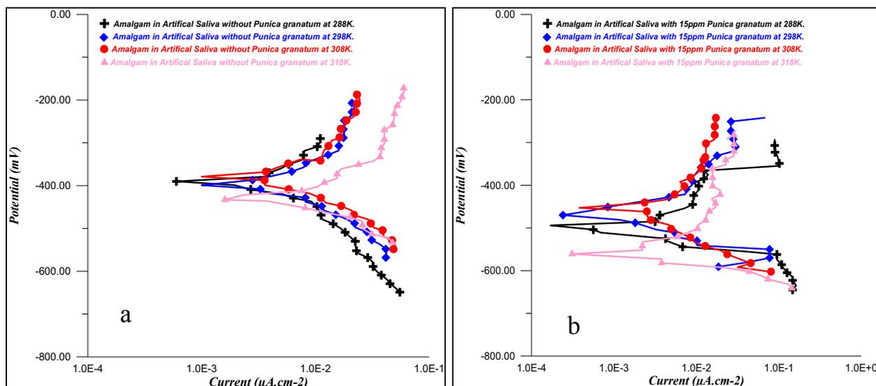
**Figure 1:** The polarization curve of amalgam in artificial saliva a) without inhibitor and b) with 15ppm inhibitor.
