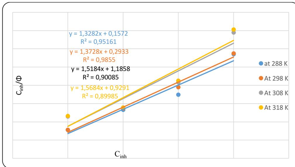
Figure 5. Langmuir isotherm plot for the adsorption of Cactus on the surface of amalgam.
