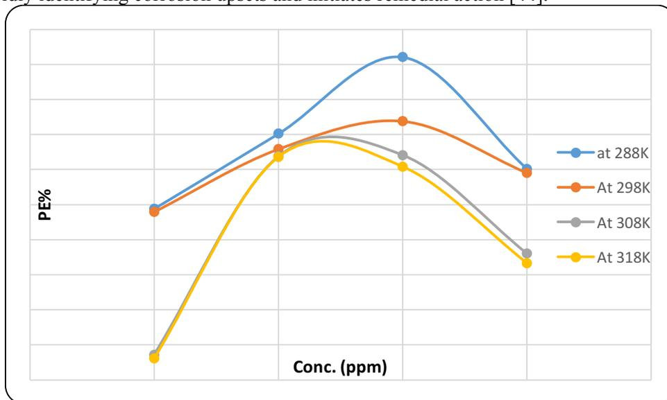
**Figure 2.** The relation between inhibitor efficiency (IE%) and inhibitor concentration in artificial saliva.
