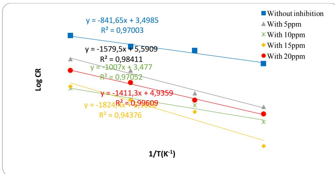
**Figure 3.** Arrhenius Plot of  $\log i_{corr}$  Versus  $1/T$  for the corrosion of amalgam in artificial saliva solution in absence and presence of various (P.g.e) concentrations.
