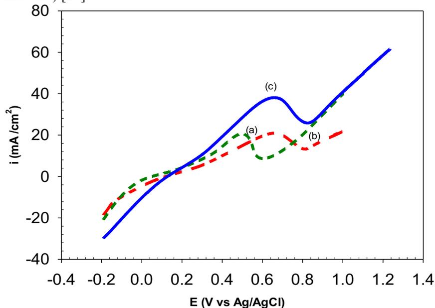
**Fig 4:** Anodic branch of cyclic voltammogram for ethanol oxidation in alkaline media at scan rate 50mV/s on Ag/C electrode prepared by double – pulse electrodeposition technique: Nucleation potential -1070 mV, Nucleation time 800ms, Growth time 90 sand different Growth potential (a)-220,(b)-320&(c)-450 mV(vs Ag/AgCl).
