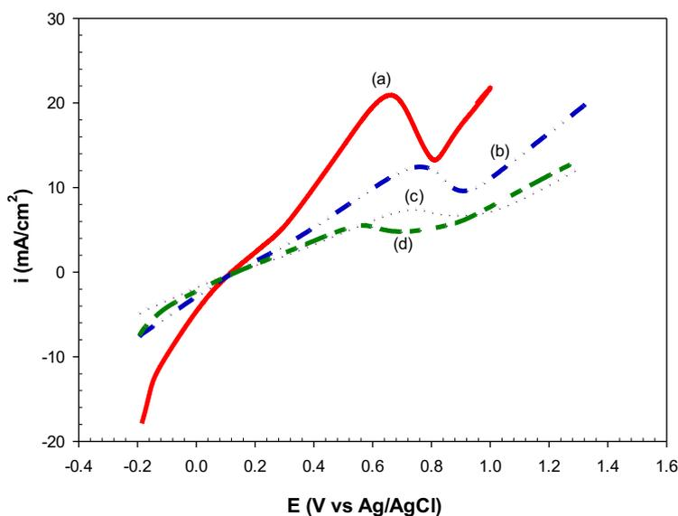
**Fig 3:** Anodic branch of cyclic voltammogram for ethanol oxidation in alkaline media at scan rate 50mV/s on Ag/C electrode prepared by double – pulse electrodeposition technique: Nucleation potential -1070 mV, Nucleation time 800ms, Growth potential -320 mV, and different Growth time (a) 90, (b) 180, (c) 360 & (d) 500s
