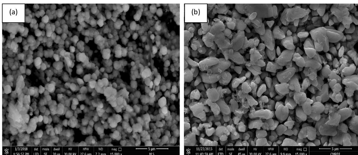
**Fig. 9:** FESEM images of Ag/C catalyst prepared by (a) double pulse and (b) pulsed current techniques
