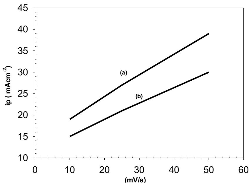
**Fig. 6:** The relation between anodic peak current densities and scan rates for Ag/C electrode prepared by (a) double-pulse, (b) pulsed current techniques at corresponding optimum condition for ethanol oxidation in alkaline media.
