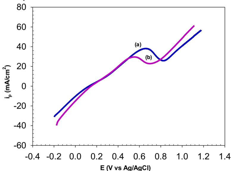
**Fig 5:** Anodic branch of cyclic voltammogram for ethanol oxidation in alkaline media at scan rate 50mV/s on Ag/C electrode prepared by (a) double – pulse, (b) pulsed current, electrodeposition techniques at corresponding optimum conditions.
