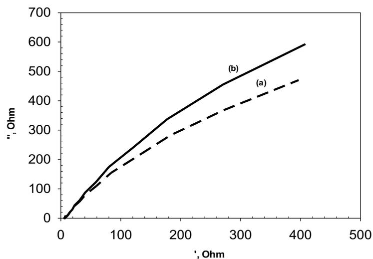
**Fig.7:** Nyquist plot on Ag/C electrode prepared by (a) double-pulse and (b) pulsed techniques at corresponding optimum conditions for ethanol oxidation in alkaline media (frequency:10kHz - 0.1 Hz, potential 500 mVAg/AgCl, amplitude :0.01 V)
