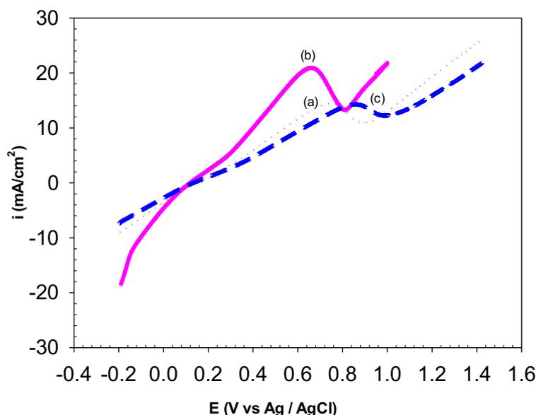
**Fig 1** : Anodic branch of cyclic voltammogram for ethanol oxidation in alkaline media at scan rate 50mV/s on Ag/C electrode prepared by double pulse electrodeposition technique: Nucleation time 800ms , Growthpotential -320mV, Growth time 90s, and different nucleation potential (a) -870,(b) -1070& (c)-1550mV (vs Ag/AgCl)
