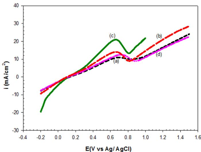
**Fig 2:** Anodic branch of cyclic voltammogram for ethanol oxidation in alkaline media at scan rate 50mV/s on Ag/C electrode prepared by double – pulse electrodeposition technique: Nucleation potential -1070 mV, Growth potential-320 mV, Growth time 90s, and different Nucleation time (a) 100, (b) 400,(c) 800 & (d)1000ms
