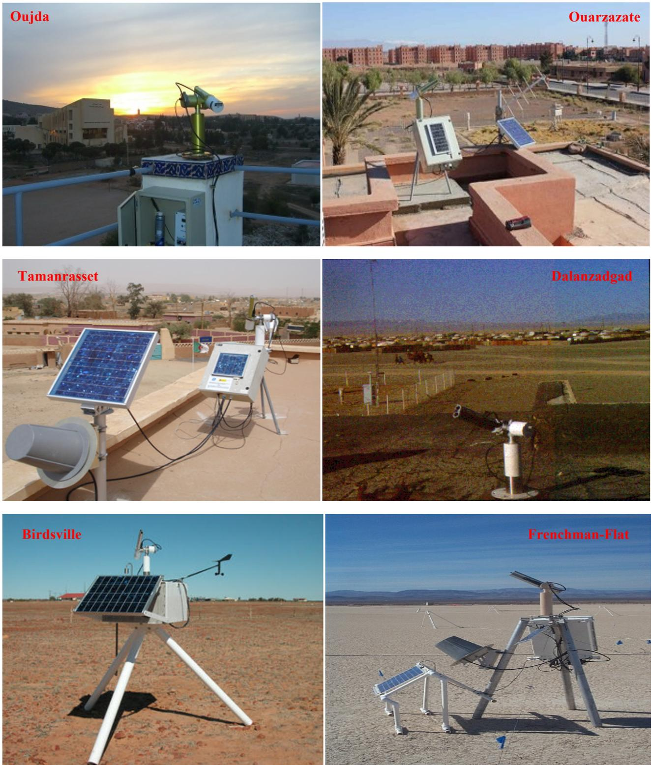
**Figure 2:** Solar photometers CIMEL CE-318 installed at the six sites
