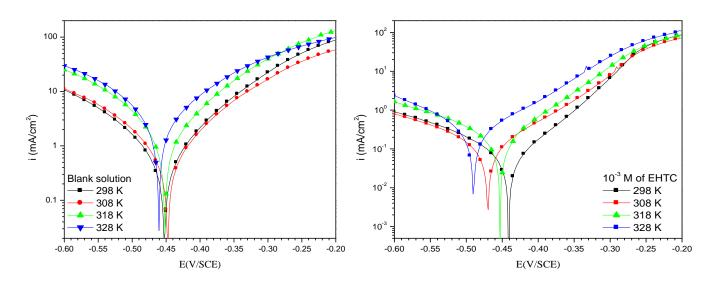
**Figure 7:** Potentiodynamic polarization curves for carbon steel in 1.0 M HCl at different temperatures.
