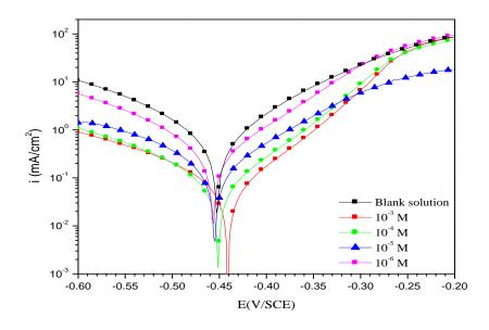
Figure 3: Potentiodynamic polarization curves for carbon steel in 1.0 M HCl containing different concentrations of EHTC.
