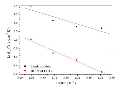
**Figure 10**: Transition-state plots for carbon steel in 1.0 M HCl in the absence and presence of 10<sup>-3</sup> M of EHTC at different temperatures.
