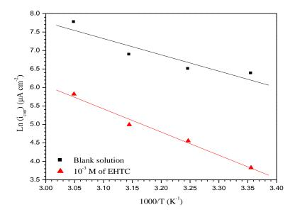
**Figure 9:** Arrhenius plots for carbon steel in 1.0 M HCl in the absence and presence of 10<sup>-3</sup> M of EHTC at different temperatures.
