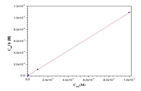
Figure 6: Langmuir adsorption isotherm plot for carbon steel in 1.0 M HCl at different concentrations of EHTC.
