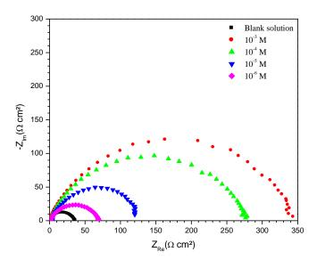
Figure 4: Nyquist plots for carbon steel in 1.0 M HCl in the absence and presence of various concentrations of EHTC at
