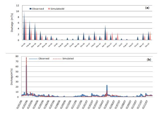
Figure 5: Observed vs simulated monthly (a) and daily (b) discharge after manual calibration at the Souk Elhad flow gauge
