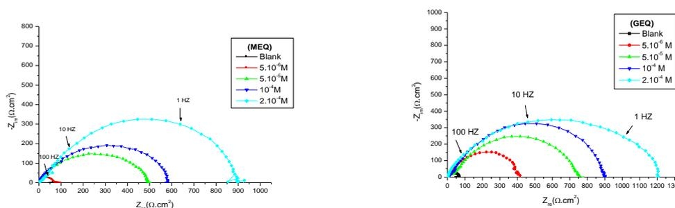
**Figure 3:** Nyquist diagrams of iron in 1M HCl without and with addition of different concentration of: (MEQ) and (GEQ)
