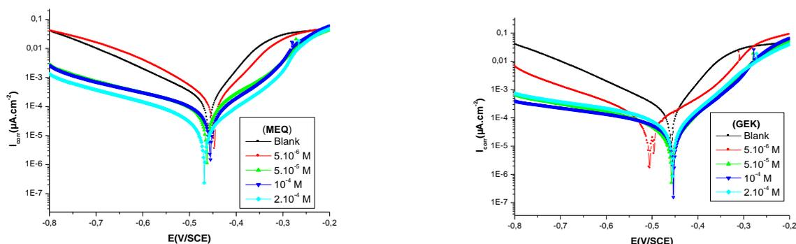
**Figure 2:** Polarization curves of iron in 1M HCl in absence and presence of different concentrations of: (MEQ) and (GEQ)
