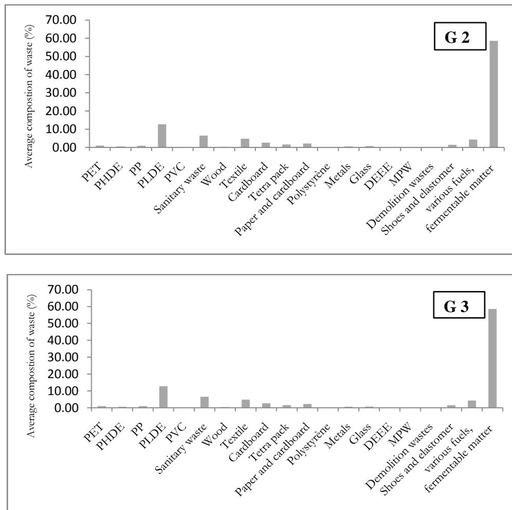
**Figure 5:** Wastes composition: (G2) Fraction between 80-250mm (G3) fraction better than 250 mm
