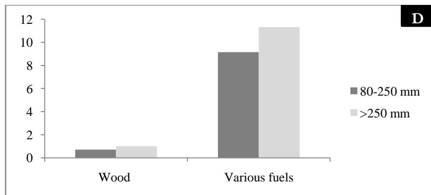
**Figure7:** Combustibles fractions distribution depending on the particle size
