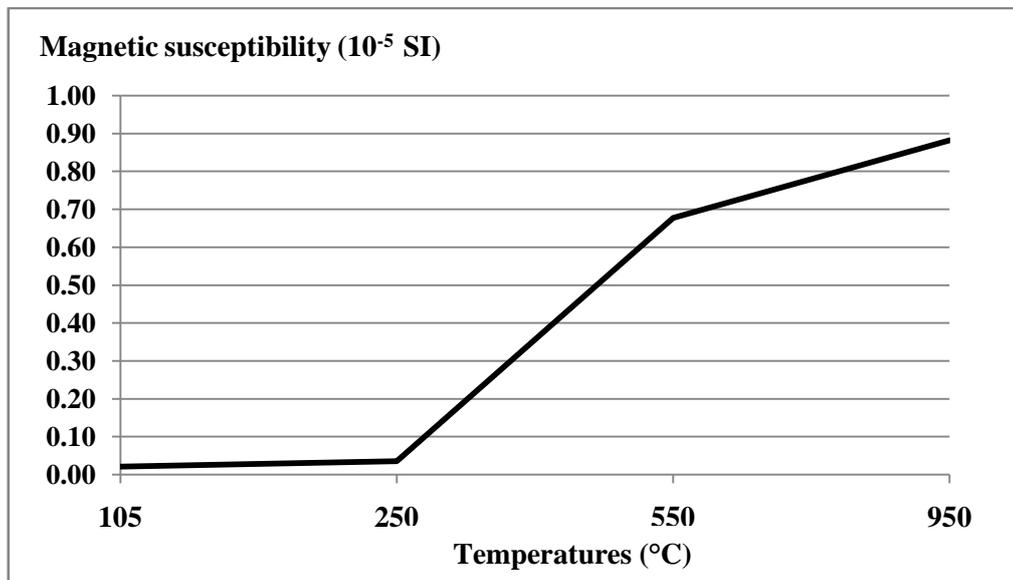
**Figure 2:** Variation of magnetic susceptibility according to the calcination temperatures
