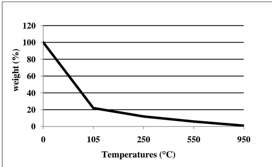
**Figure 1:** Weight loss of sewage sludge during the calcination at 105°C – 950°C
