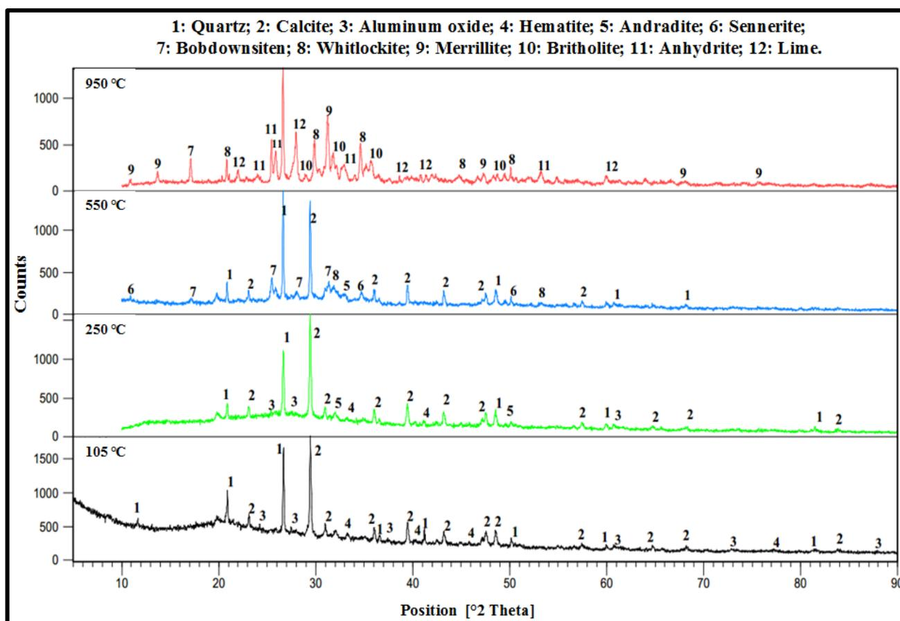
Figure 4: X-ray diffraction diagrams of sewage sludge ashes
