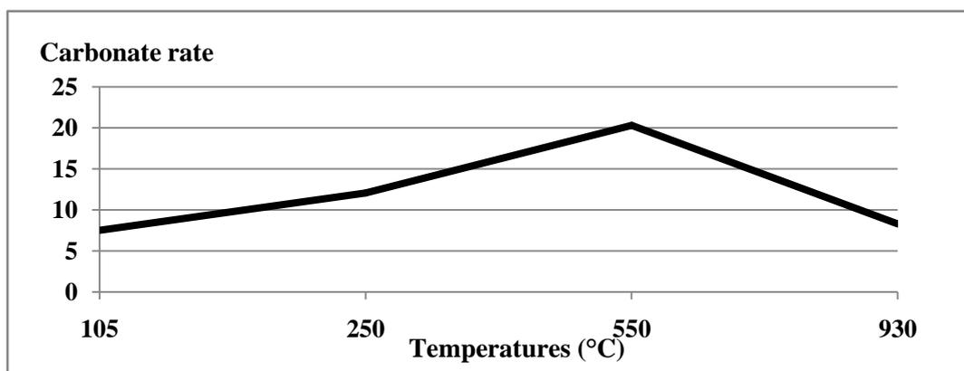
**Figure 3:** Variation of carbonate calcium according to the calcination temperatures.
