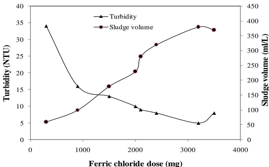
**Figure 1b:** Evolution of turbidity and sludge volume depending on the dose of  $\text{FeCl}_3$
