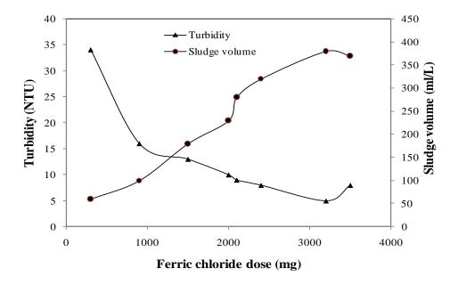
Figure 1b: Evolution of turbidity and sludge volume depending on the dose of FeCl<sub>3</sub>
