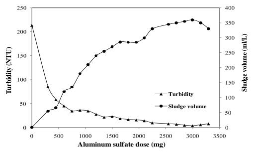
Figure1a: Evolution of turbidity and sludge volume depending on the dose of Al<sub>2</sub>(SO<sub>4</sub>)<sub>3</sub>
