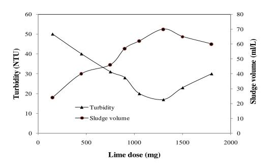
Figure 1c: Evolution of turbidity and sludge volume depending on the dose of Ca(OH)<sub>2</sub>
