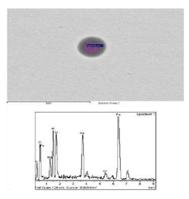
Figure 7: Typical inclusion on the refining phase (calcium-silicate) [20, 21]
