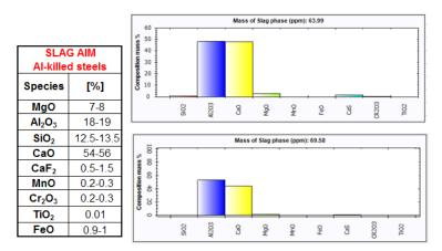
**Figure 2:** Composition aim slag (left) obtained from thermodynamic calculations (using ThermoCalc). Composition and mass inclusions in Al-killed steel computed using software developed by CSM utilizing a "thermodynamic core" based on Thermo-Calc
