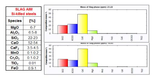
**Figure 6:** Slag aim composition (left) obtained from thermodynamic calculations (using Thermo-Calc). Composition and mass inclusions in Al-killed steels calculated using software developed by CSM employing a "thermodynamic core" based on Thermo-Calc
