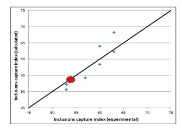
Figure 8: Representation of inclusions capture index for the aim slag (Si-killed)
