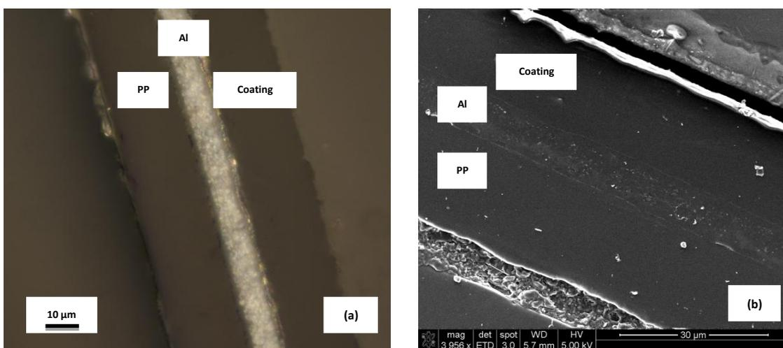
**Figure 1:** Metallised plastic structure, a) Optical microscopy and b) scanning electronmicroscopy
