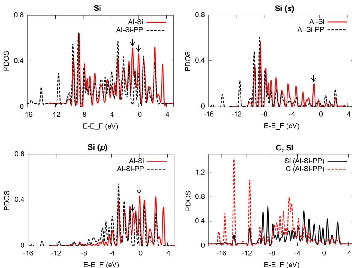
**Figure 6:** PDOS of Si in Al-Si-PP and in Al-Si. (a) total, (b) s orbitals, (c) p orbitals; and (d) PDOS of Si and the C in PP attached to Si in Al-Si-PP structure. Fermi level is set to zero.
