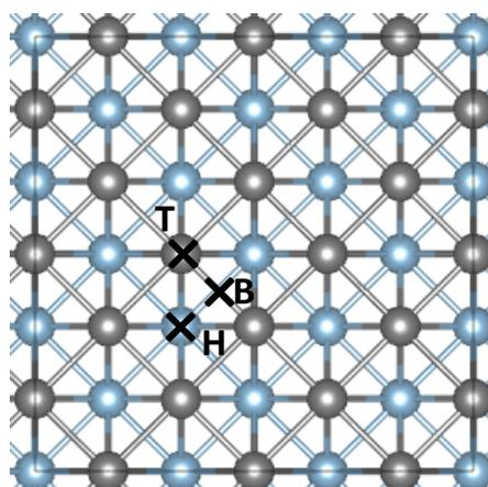
**Figure 4:** The structure of Al (100) surface of FCC Al lattice from the top view. T, B and H show the position of the top, bridge, and hollow absorption sites, respectively. Grey shows the surface atoms, while other Al atoms are shown in blue.
