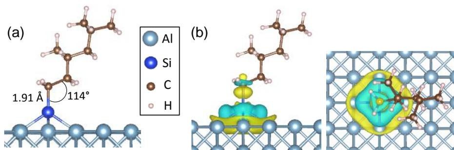
**Figure 5:** (a) Relaxed structure of PP deposited on the Al (100) surface on Si in the hollow site, (b) charge density difference isosurface of the Al-PP interface from side view (left) and top view (right). Blue corresponds to charge depletion and yellow to charge accumulation. The isosurface value is  $5 \times 10^{-3} \text{ e}/\text{\AA}^3$ .
