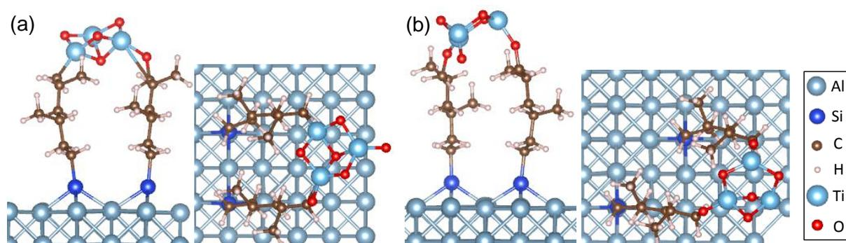
**Figure 7:** Relaxed structure of Al (100)-Si-PP-Ti<sub>3</sub>O<sub>6</sub> from side view (left) and top view (right) (a) the minimum energy structure; (b) structure with larger Si-Si distance
