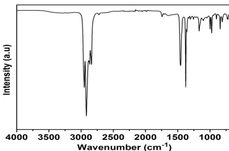
**Figure 2:** FTIR spectrum of metallised plastic
