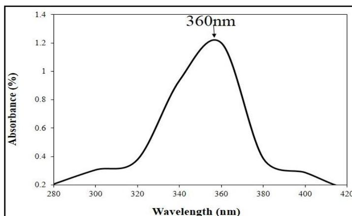
Figure 2: UV-visible spectrum of copper oxide nanoparticles synthesized.
