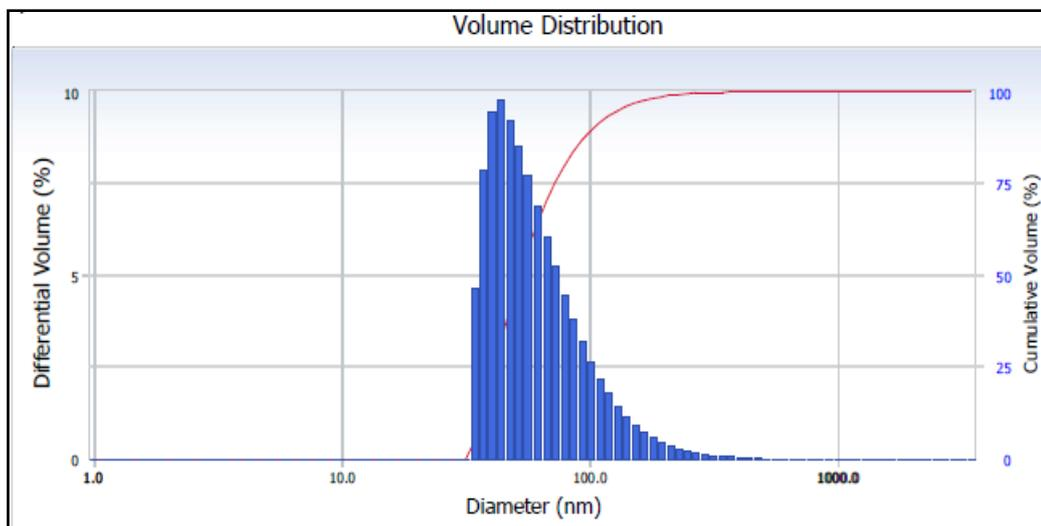
**Figure 4:** Particle size distribution of synthesized copper oxide nanoparticles.
