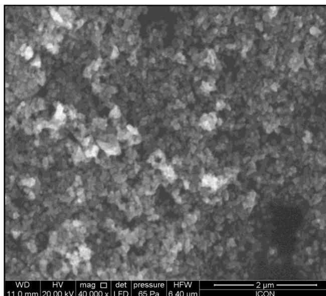
**Figure 6:** SEM image of the synthesized copper oxide nanoparticles.
