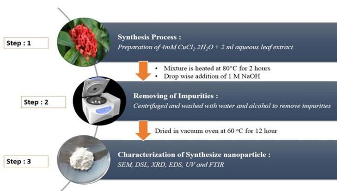
**Figure 1:** Graphical representation for formation of copper oxide nanoparticles.
