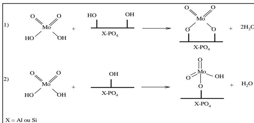
1- Reaction of a molybdenum atom with two OH groups to form an acid site of Lewis,
