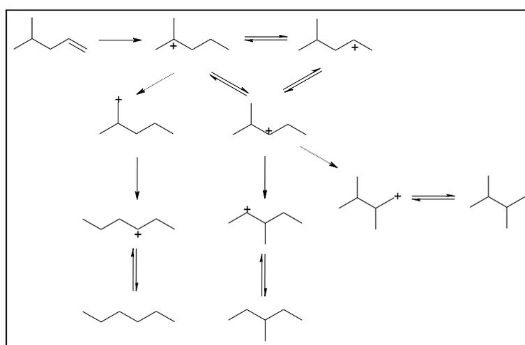
**Figure 5:** Isomerization of the 4M1Pene in 23DMB, 3MP and n-Hex by an acid mechanism by formation of carbonium ions according to Garin and Coll, [40]
