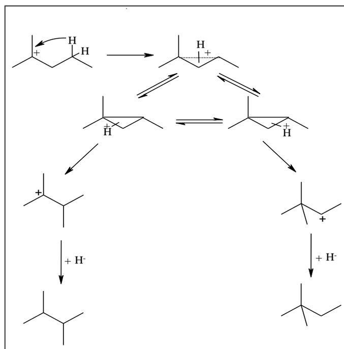
**Figure 7:** Mechanism with cyclopropanic complexes
