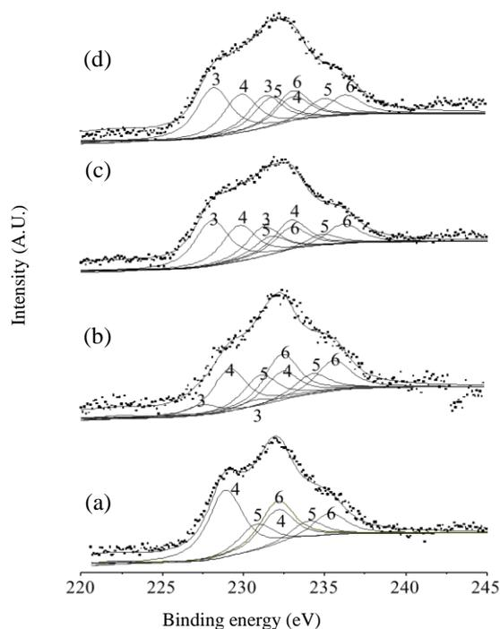
**Figure 3 :** The XPS of MoAlP 3d following different times of in-situ treatments with H<sub>2</sub> at 450°C: (a) 2h, (b) 4h, (c) 12h, (d) 17h.
