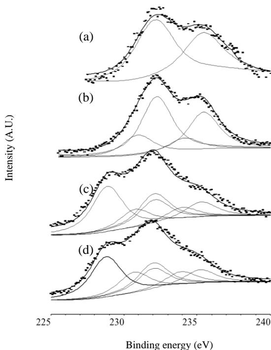
**Figure 2 :** The XPS of MoAlP 3d following different temperatures of in-situ treatments with H<sub>2</sub> for 2hour: (a) before any treatment, (b) 350°C, (c) 450°C, (d)
