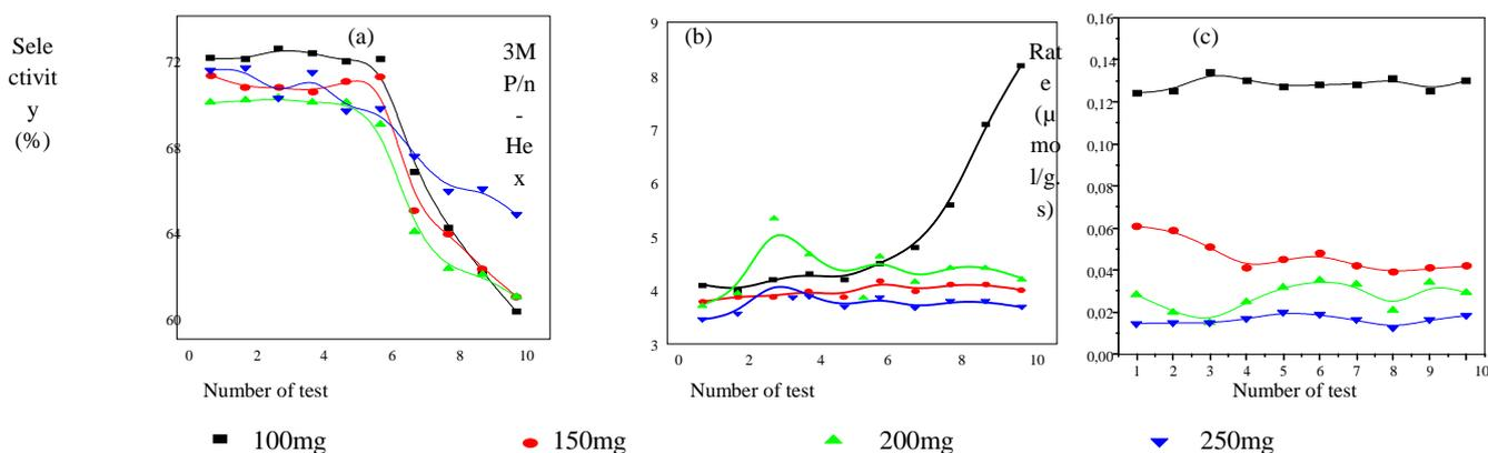
**Figure 4** : Evolution of the selectivity, the ratio of the 3MP/n-Hex and rate of reaction with the number of catalytic testing at 380°C on different masses of catalyst in the isomerization of 2MP
