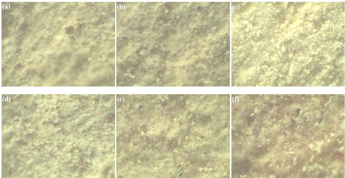
**Figure 8:** OM images (100 times magnified) of fractured geopolymers result for heated kaolinitic clay at 700 °C and different base concentrations: (a) geopolymer specimen synthesized by KOH 8 M, (b) geopolymer specimen synthesized by KOH 13 M, (c) geopolymer specimen synthesized by KOH 15 M, (d) geopolymer specimen synthesized by NaOH 8 M, (e) geopolymer specimen synthesized by NaOH 13 M, (f) geopolymer specimen synthesized by NaOH 15 M
