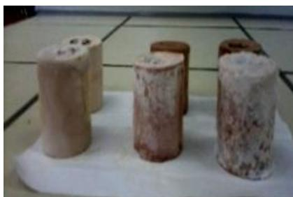
**Figure 6:** Formation of the white carbonate on surface of specimens known as efflorescence which usually induced degradation of binder
