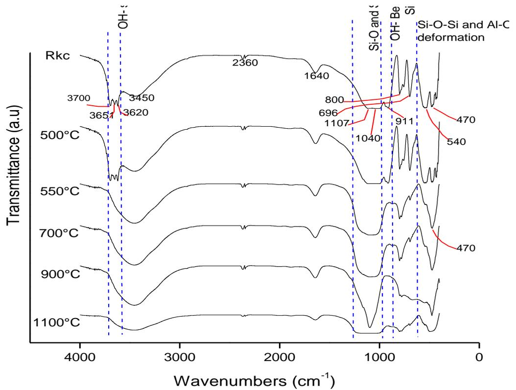
**Figure 2:** IR spectra of heat-treated and raw kaolinitic clay (Rkc) at different temperatures for 2 h.
