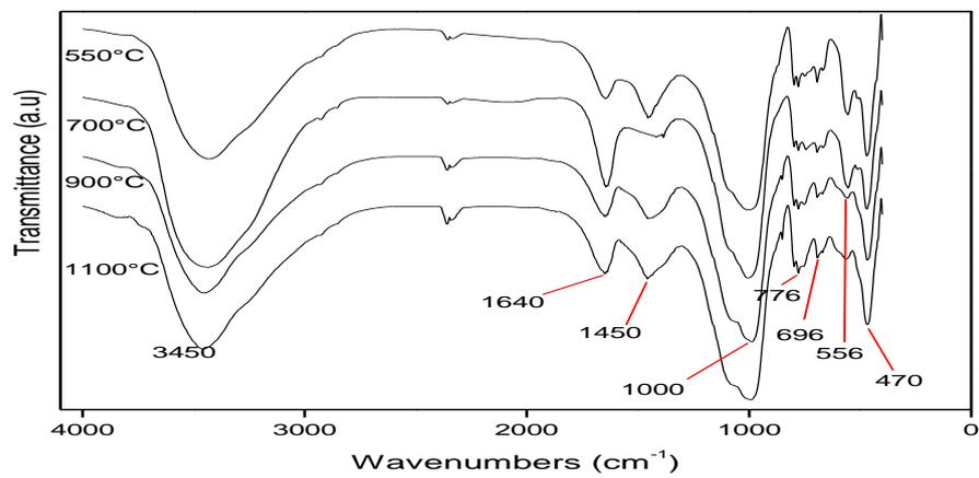
**Figure 15:** IR spectra patterns of samples obtained by mixing the clay fractions calcined at 550, 700, 900 and 1100 °C with 15-NaOH solutions
