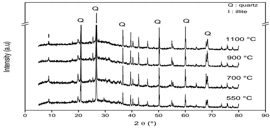
**Figure 9:** XRD patterns on calcined clay at 550, 700, 900 and 1100 °C and mixed with KOH (15 M)
