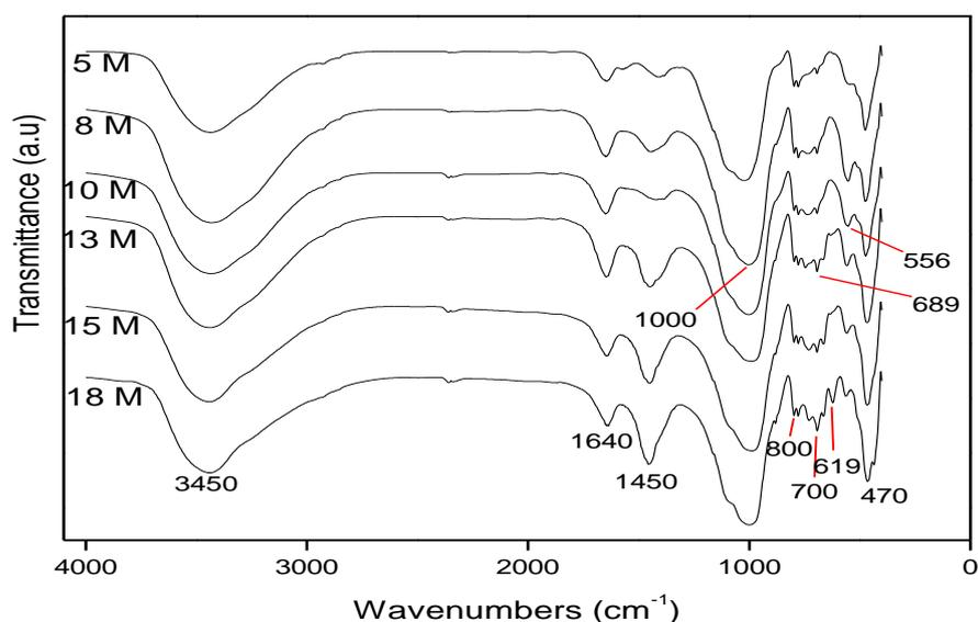
**Figure 17:** IR spectra of Samples obtained with the kaolinitic clay calcined at  $700\text{ }^{\circ}\text{C}$  and different NaOH concentrations
