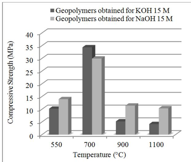
**Figure 4:** Geopolymer compressive strength result for different heated temperatures of kaolinitic clay and KOH and NaOH 15 M (Three cylinders of each sample were tested, averaging the experimental values obtained).
