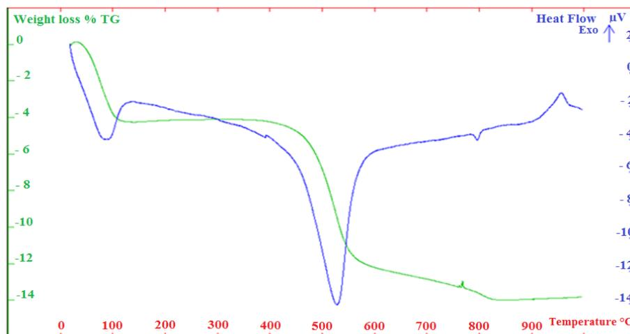
**Figure 3:** Thermogravimetric (TGA, green curve) and differential thermal analysis (DTA, blue curve) of the raw kaolinitic clay.
