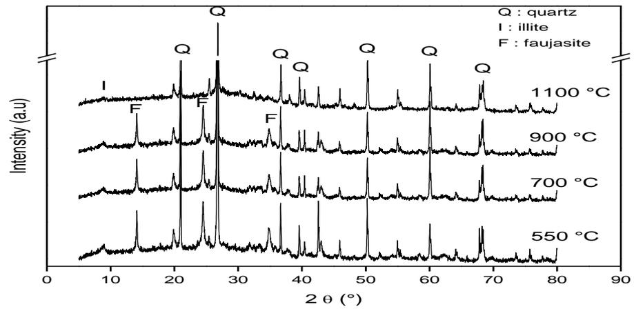
**Figure 10:** XRD patterns on calcined clay at 550, 700, 900 and 1100 °C and mixed with KOH (15 M)
