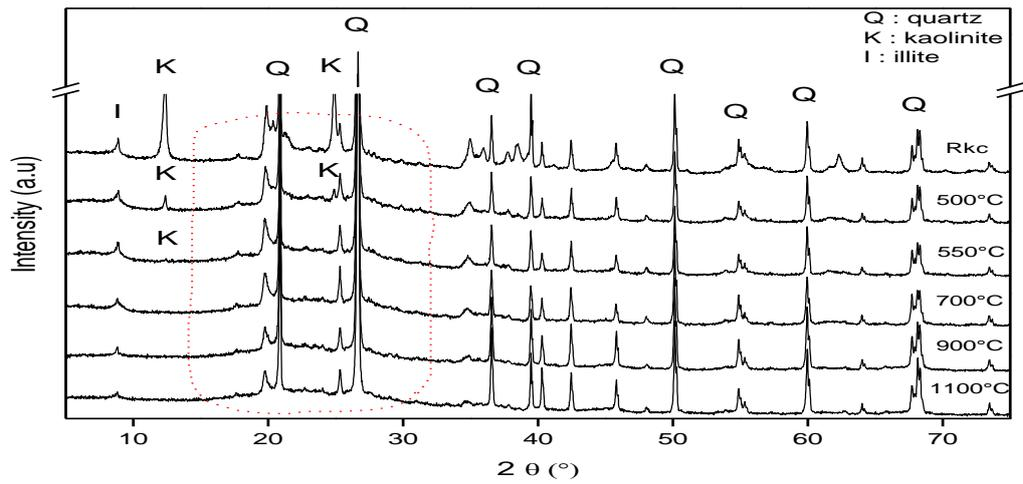
**Figure 1:** X-ray diffraction patterns on heat-treated and raw kaolinitic clay (Rkc) at different temperatures for 2 h
