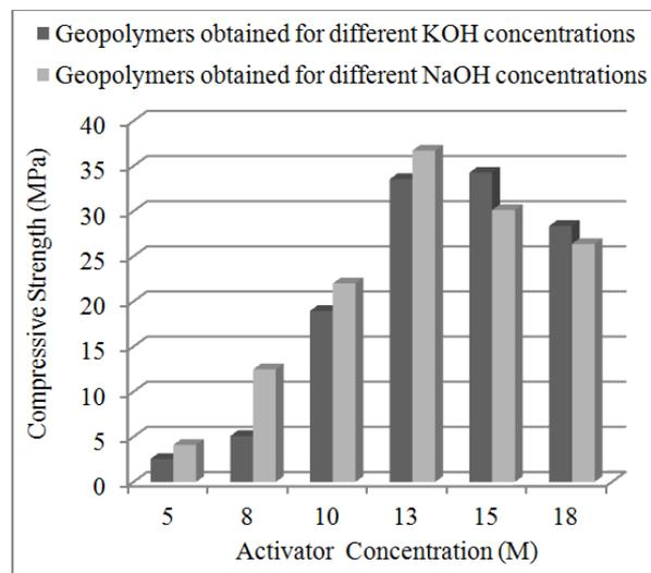
**Figure 5:** Geopolymer compressive strength result for heated kaolinitic clay at  $700^\circ\text{C}$  and different base concentrations (Three cylinders of each sample were tested, averaging the experimental values obtained).
