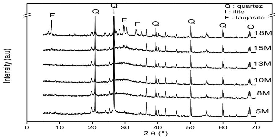
**Figure 11:** XRD patterns on calcined clay at 700°C and mixed with different KOH concentrations
