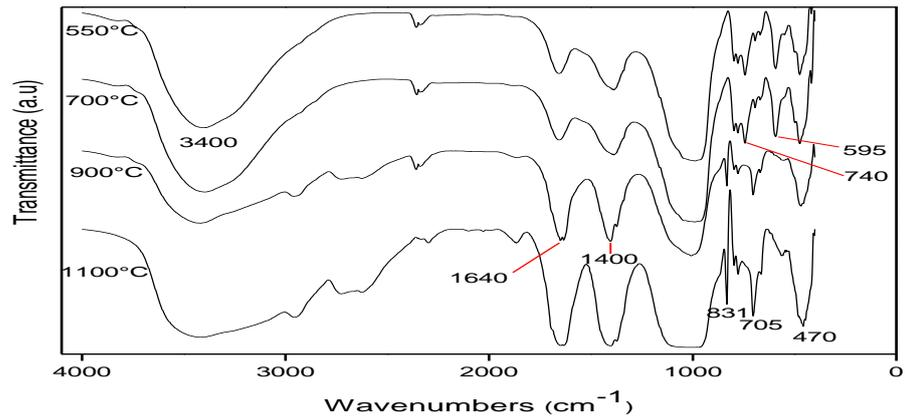
**Figure 14:** IR spectra patterns of samples obtained by mixing the clay fractions calcined at 550, 700, 900 and 1100 °C with 15M-KOH solutions
