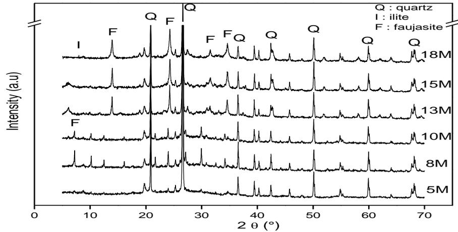
**Figure 12.** XRD patterns on calcined clay at 700 °C and mixed with different NaOH concentrations
