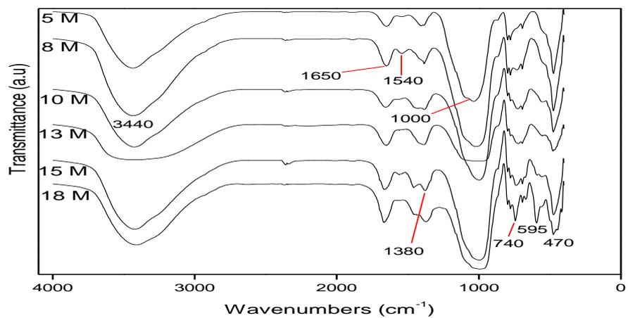
**Figure 16.** IR spectra of Samples obtained with the kaolinitic clay calcined at 700 °C and different KOH concentrations
