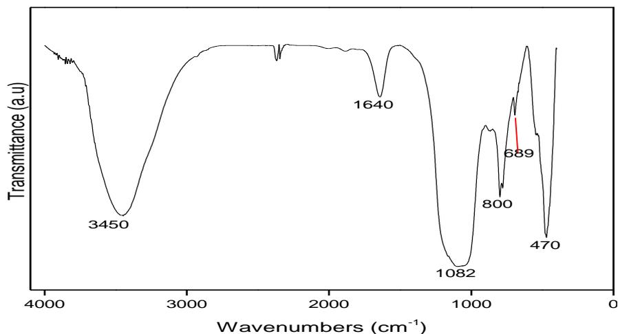
**Figure 13:** IR spectra of metakaolin (calcined kaolinitic clay at 700 °C)
