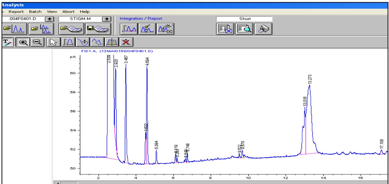
**Figure 2:** Example of chromatogram of a sample of BTX (RT (benzene) = 2.9 min, RT (toluene) = 3.5 min, RT (m-xylene) = 4.5 min, RT (p-xylene) = 4.6 min and RT (o-xylene) = 5.1 min)
