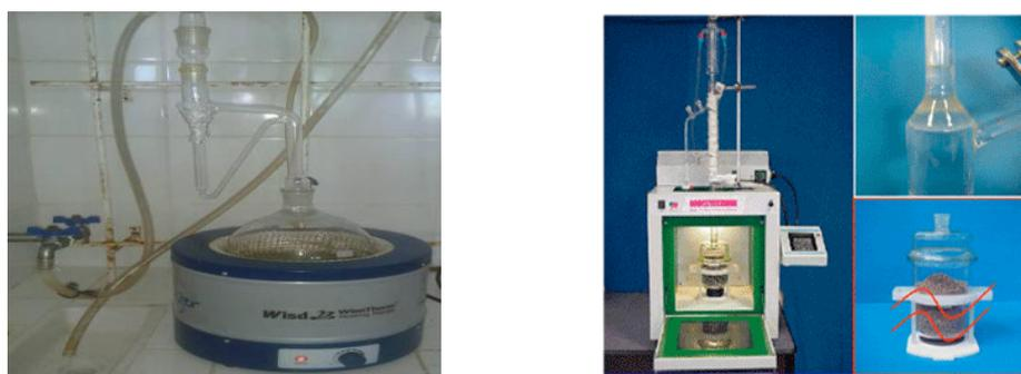
**Figure 1:** Montage the extraction of essential oil: Classical hydrodistillation (left) and microwave-assisted hydrodistillation (right).
