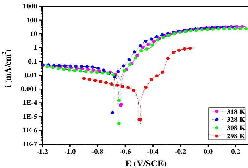
**Fig. 5:** Potentiodynamic polarization curves of tinplate in 3%NaCl (pH = 2) in the presence of 0.5 g/L of NEO at various temperatures.
