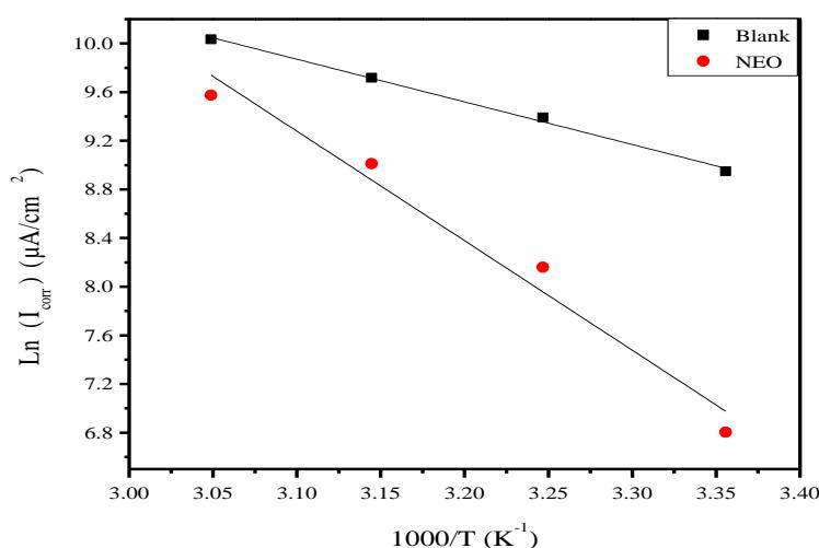
**Fig. 6:** Arrhenius plots of tinplate in 3% NaCl (pH = 2) in the absence and presence of 0.5g/L of NEO.
