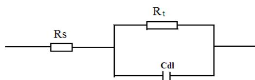
**Fig. 2:** Generally accepted equivalent circuit for metal/solution interface.
