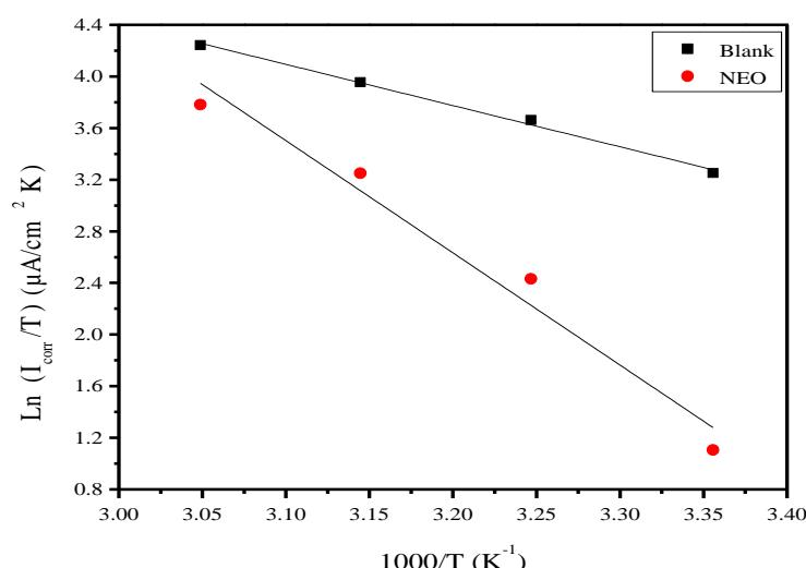
**Fig. 7:** Transition Arrhenius plots of tinplate in 3% NaCl (pH = 2) in the absence and presence of 0.5 g/L of NEO.
