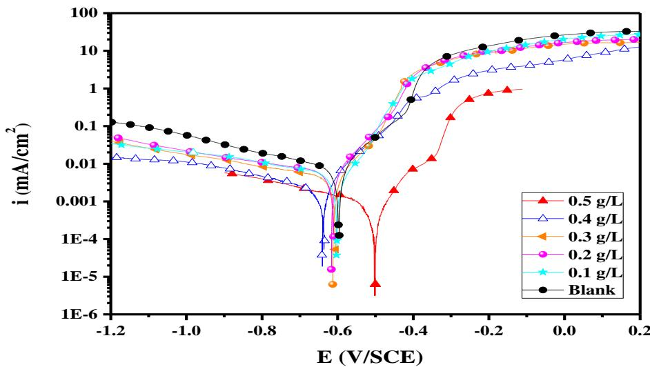
**Fig. 1:** Potentiodynamic polarisation curves of tinplate in 3% NaCl, for various concentrations of NEO at 298 K
