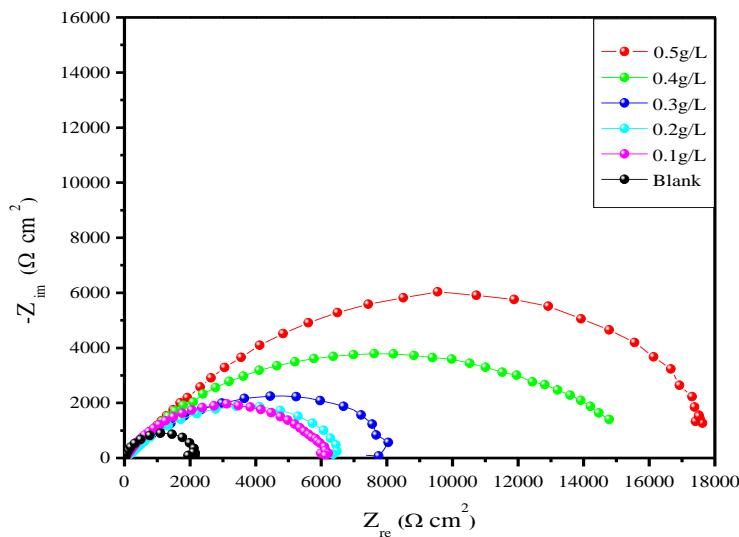
**Fig. 3:** Nyquist diagrams for tinplate electrode in 3% NaCl at pH = 2 at various concentrations of NEO at 298K.
