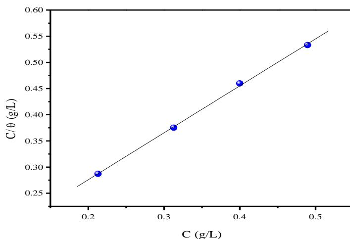
**Fig. 8:** Langmuir adsorption isotherm of NEO on tinplate surface in 3% NaCl (pH = 2) solution at 298 K.
