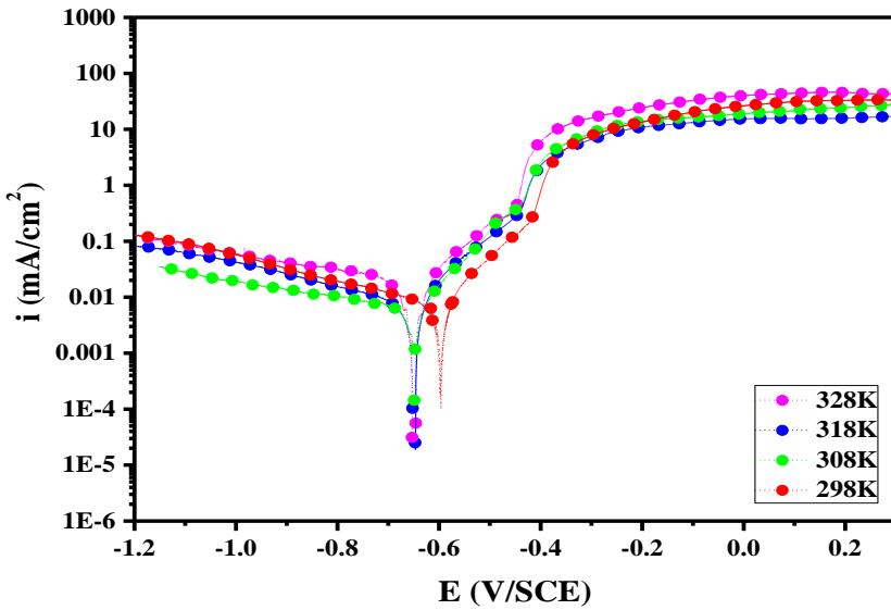
**Fig. 4:** Potentiodynamic polarization curves of tinplate in 3% NaCl (pH = 2) without NEO at various temperatures
