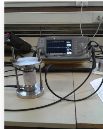
Figure 4: Experimental device for measuring ultrasound
