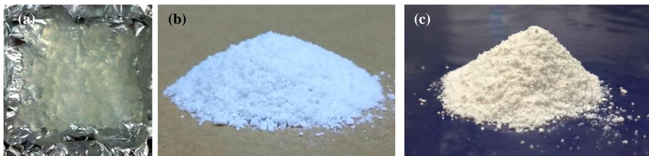
**Figure 2:** Macrostructural images of (a) as-prepared gel, (b) as-prepared xerogels, and (c) as-prepared silica powder derived from CCA burned at 600 °C.
