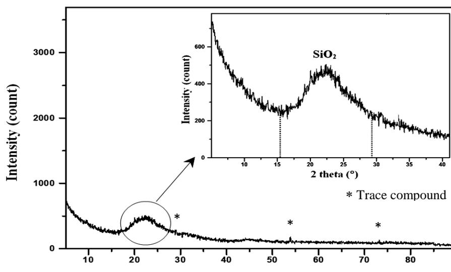
**Figure 3:** XRD pattern of as-prepared silica powder derived from CCA burned at 600 °C.
