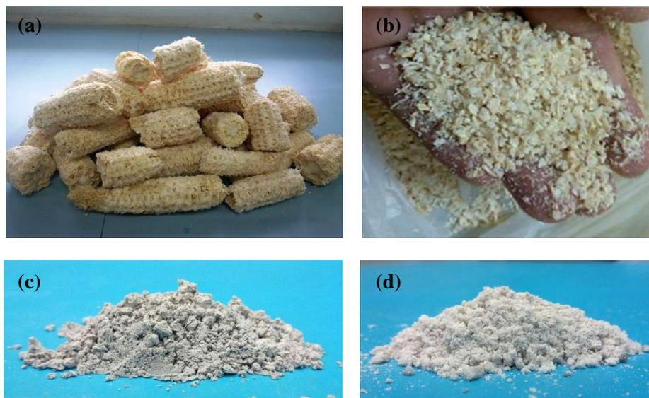
**Figure 1:** Macrostructural images of corn cob in different forms (a) dried-bulk corn cobs, (b) ground-corn cobs, (c) CCA powder burned at 600 °C, and (d) CCA powder burned at 800 °C.
