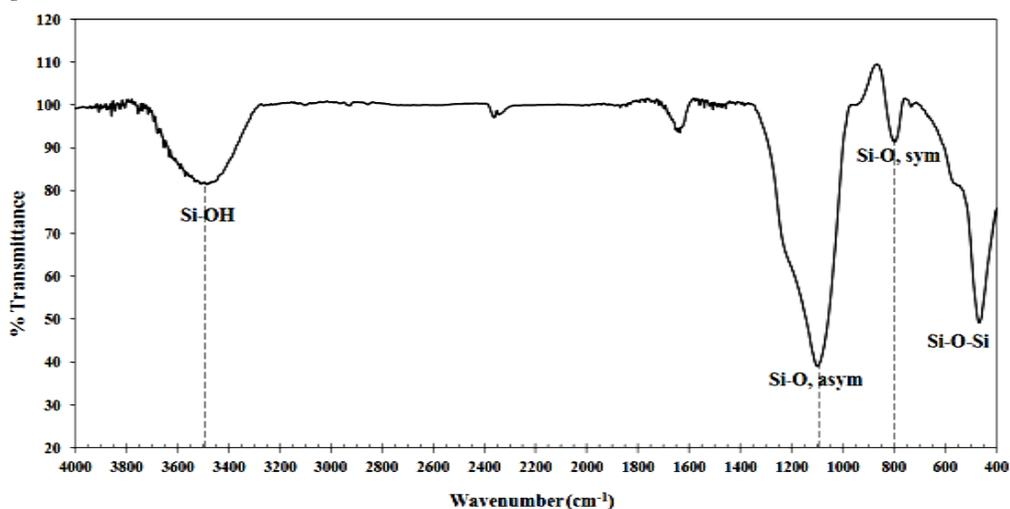
**Figure 4:** FT-IR spectrum of as-prepared silica powder derived from CCA burned at 600 °C.
