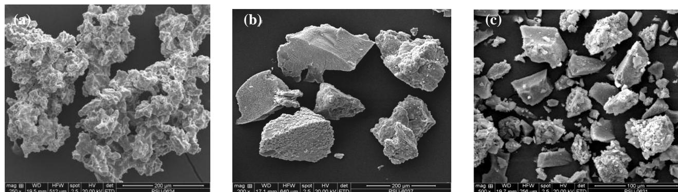
**Figure 5:** Microstructural images of (a) CCA powder burned at 600 °C, (b) as-prepared xerogels, and (c) as-prepared silica powder derived from CCA burned at 600 °C.
