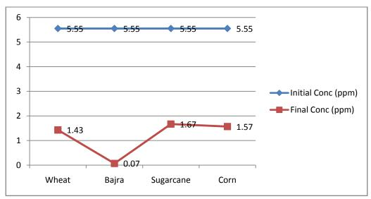
**Figure 1:** Copper removal by agro-wastes (5 ppm concentration)
