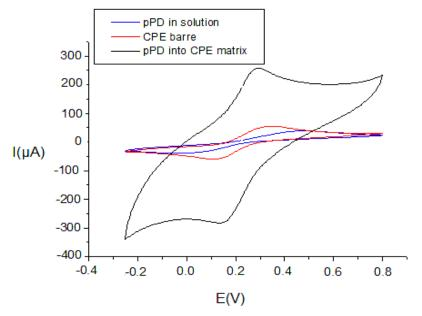
**Figure 2** Cyclic voltammogram of Fe  $(CN)_6^{3^{-/4-}}$  obtained at bare CPE, at CPE modified in surface and at CPE modified in volume by 1% of p-phenylenediamine.
