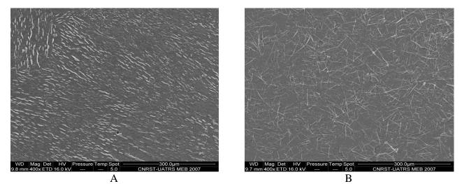
Figure 1: Morphology of CPE modified in surface (A) and CPE modified in volume (1% of p-phenylenediamine) (B)
