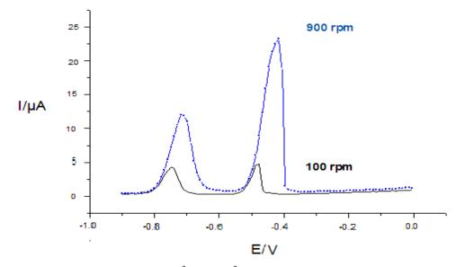
**Figure 6:** Voltammogram of 100 ppb of Cd<sup>2+</sup> and Pb<sup>2+</sup> determination at Carbone paste electrode modified in volume by poly (p-phenylenediamine), for two rotating rate 100 and 900 rpm. Condition:  $E_{dep} : -1.1V/ECS$ ,  $t_{dep} : 120$  s,  $t_{eq}$  de 30 s; Electrolyte support : HCl 0.1 mol L<sup>-1</sup>.
