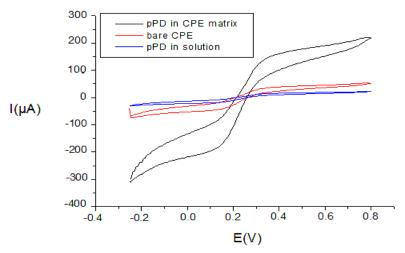
**Figure 3** Ferro/ferricyanide couple response studied by cyclic voltammetry and rotating disk electrode at the bare CPE, at the CPE modified in volume (1%) by poly (p-phenylenediamine) and at CPE modified in surface. The rotation rate and the sweep rate used in this experience are 100 rpm and 10mV/s, respectively.
