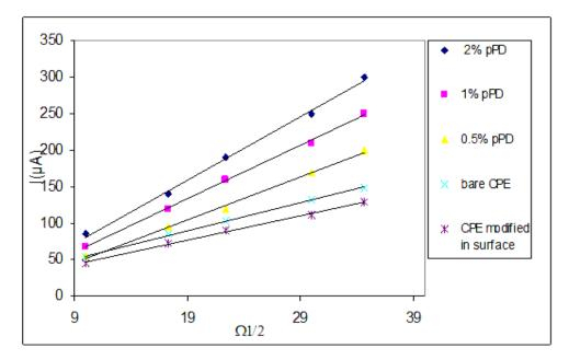
**Figure 4** Levich plots  $(i_p - \Omega^{1/2})$  obtained at different electrodes (bare CPE and modified CPEs), varying rotating rate between 100 rpm to 1200 rpm and potential from -0.4 V/ECS to 0.8 V/ECS, with a sweep rate in order to 10 mV/s.
