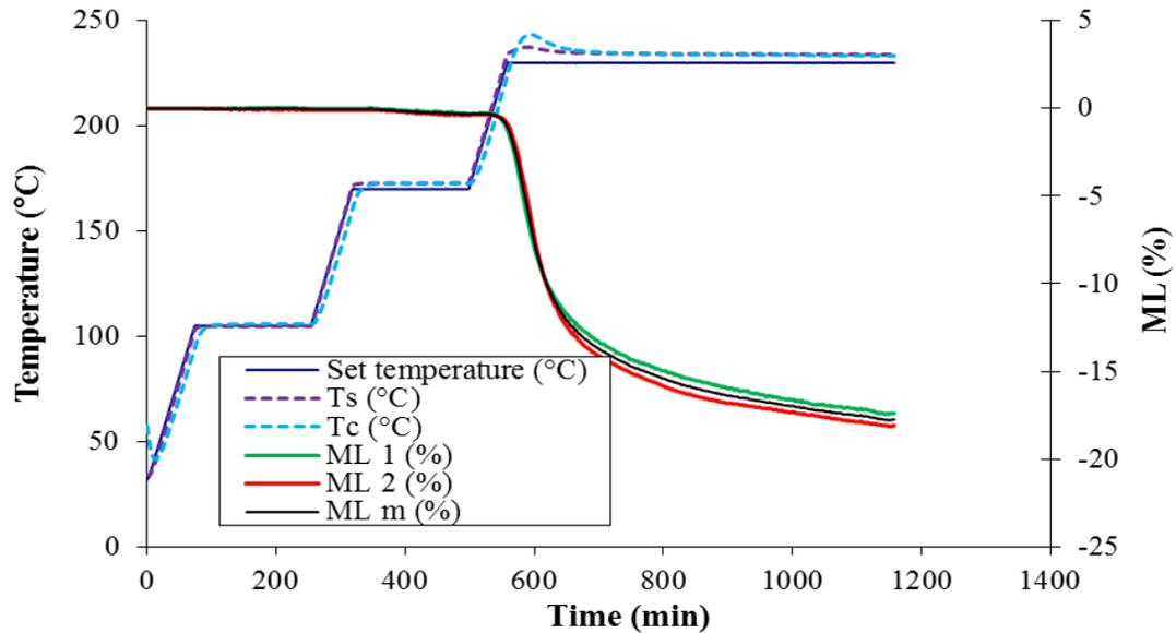
**Figure 2:** Thermo-degradation of beech wood treated at 230°C (1°C.min<sup>-1</sup>)
