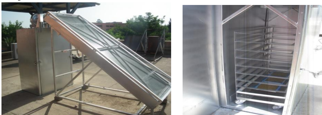
Figure 1: Convective solar dryer (LISPAM, ENS Marrakech)
