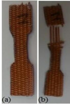
Figure 14: Samples before (a) and after (b) the tensile test.
