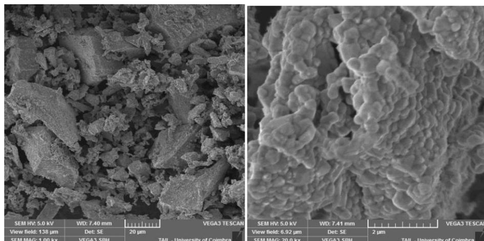
**Figure4:**SEM micrographs of  $\text{CuFe}_2\text{O}_4$  annealed at 1000°C.
