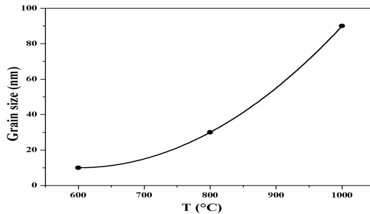
**Figure3:** Variation of grain size with annealed temperature. The curve between points is a guide to the eye.
