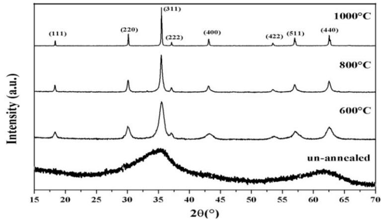
**Figure2:**XRD patterns for the annealed samples.
