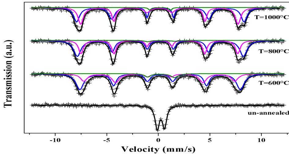
**Figure 5:** Mössbauer spectra recorded at room temperature for the un-annealed and the annealed samples at 600, 800 and 1000°C.
