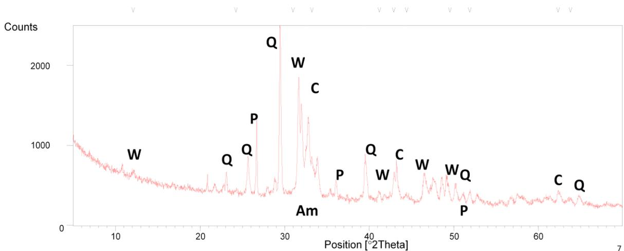
*Am: Amorphous phase; A: Anhydrite; C: Calcite; P: Portlandite; Q: Quartz; W: Witlokite.*
