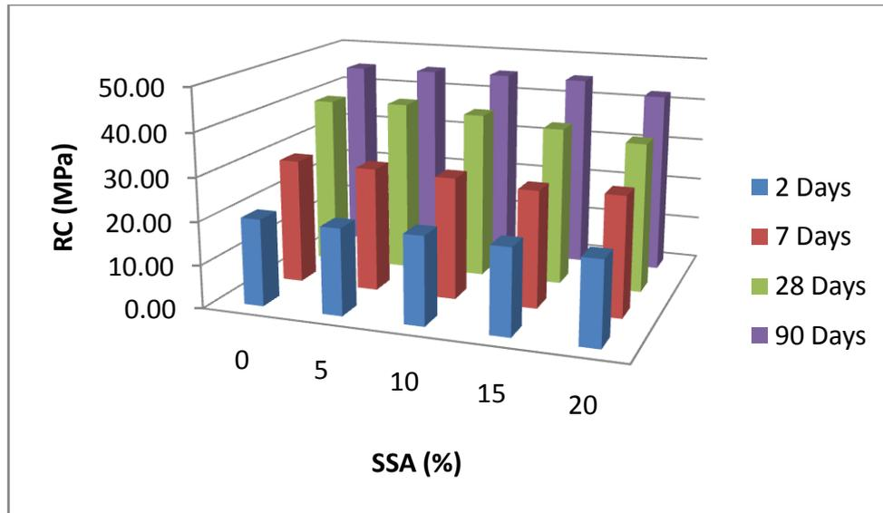
**Figure 8:** Compressive strengths of cements-SSA mixtures
