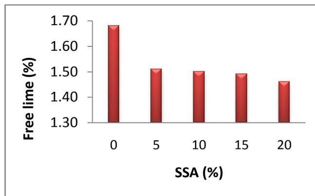
**Figure 4:** Free lime of cements-SSA mixtures
