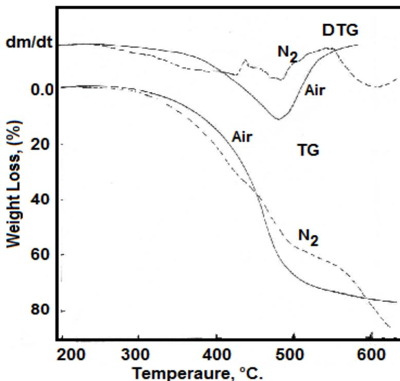
Figure 2: TG and DTG curves of Daura asphalt under air and nitrogen.
