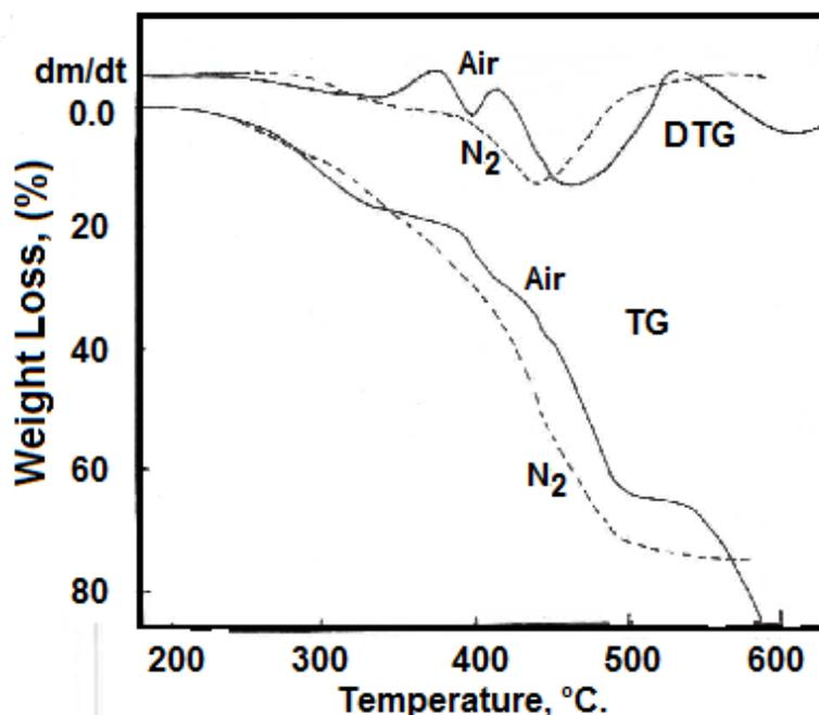
**Figure 1:** TG and DTG curves of Quayarah asphalt under air and nitrogen.
