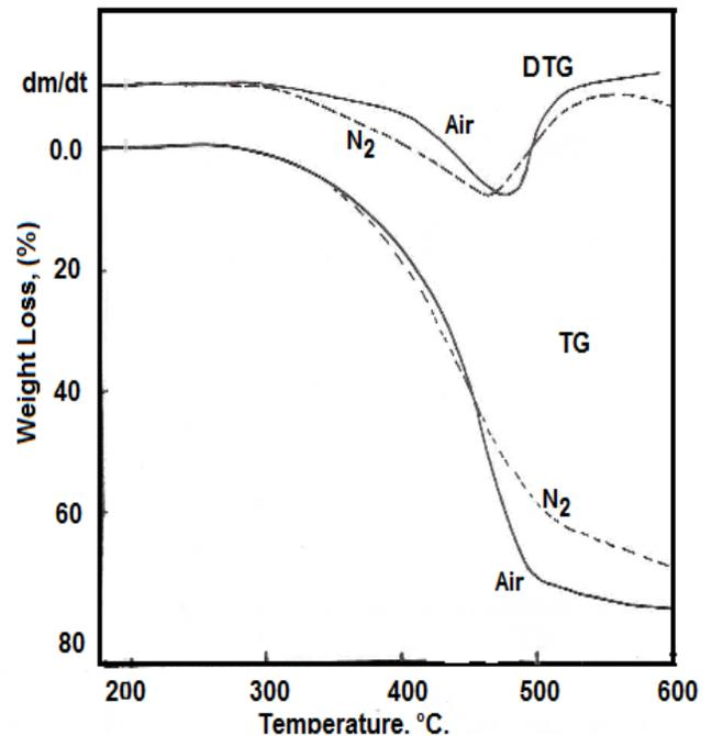
Fig. 4: TG and DTG curves of Daura asphalt after TFOT treatment under air (solid line) and nitrogen (dashed line).
