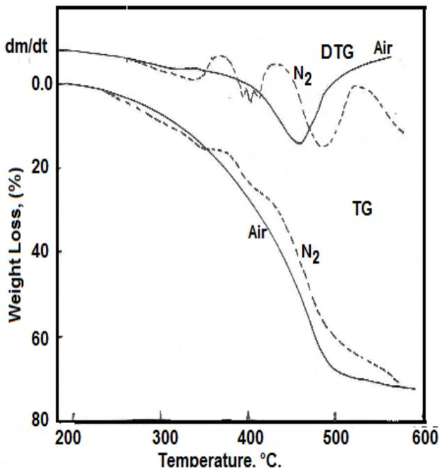
Figure 3: TG and DTG curves of Quayarah asphalt after TFOT treatment under air and nitrogen.
