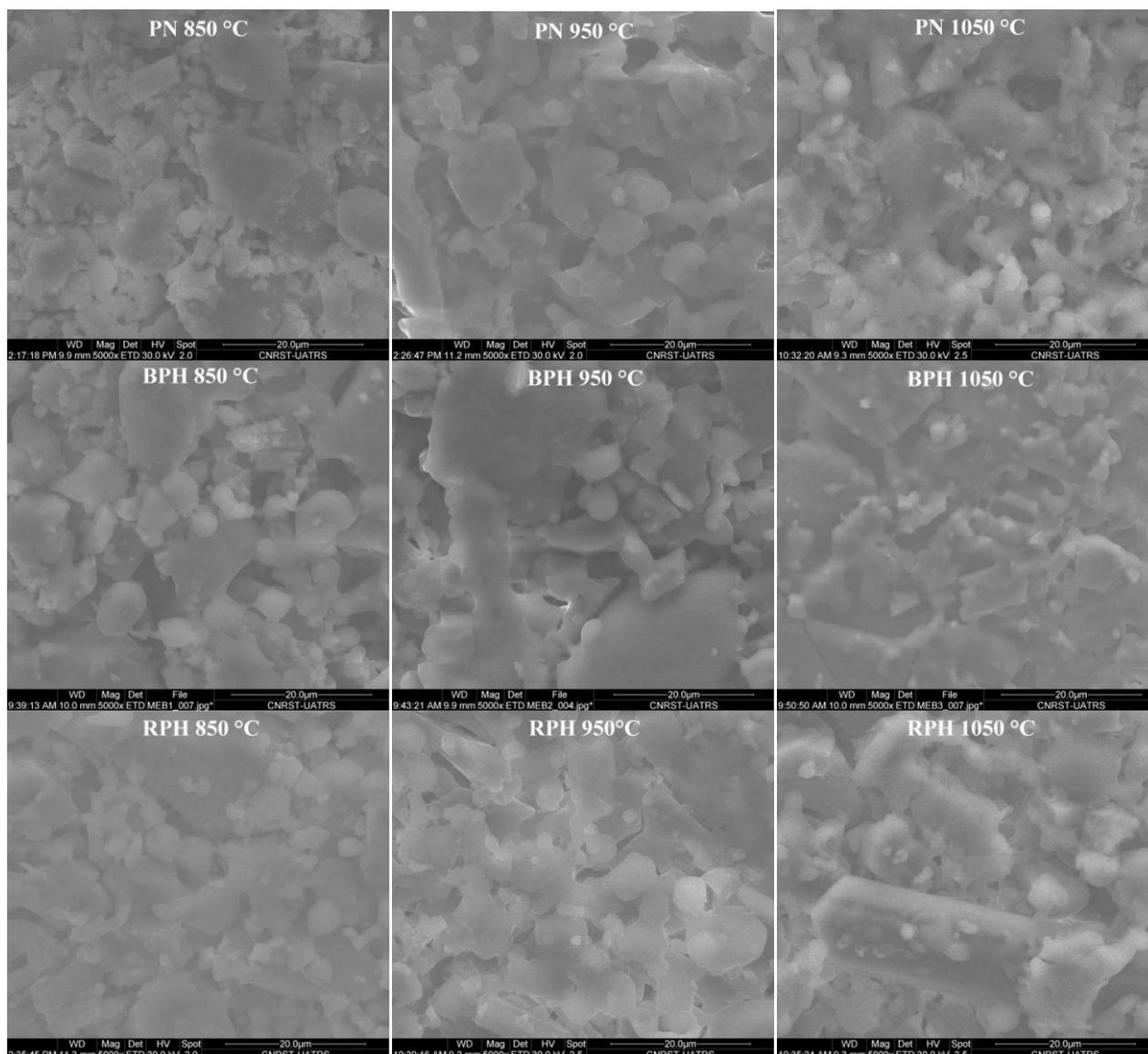
**Figure 6:** SEM images of membranes sintered at 850 °C, 950 °C and 1050 °C.
