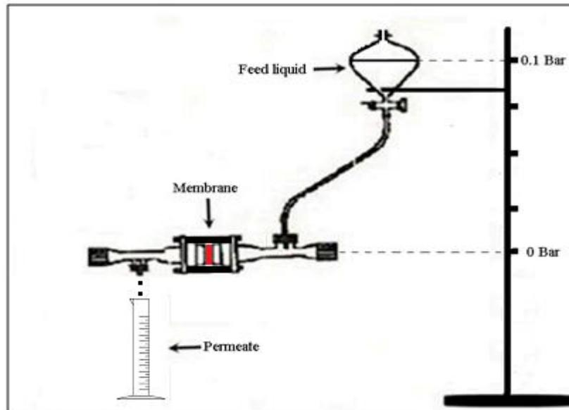
**Figure 2:** Laboratory setup for microfiltration at low pressure.
