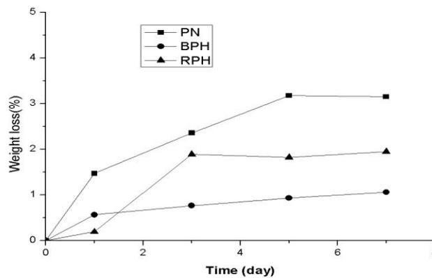
**Figure 8:** Weight loss of membranes in HCl solution at pH=1.5.
