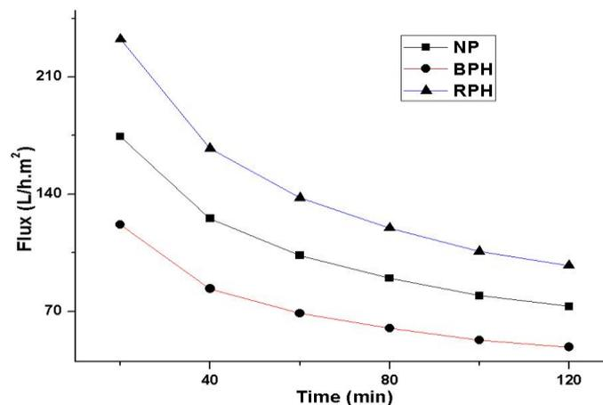
**Figure 11:** Permeate of textile effluent vs. filtration time.
