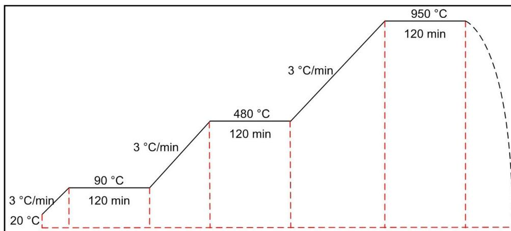
**Figure 1:** Thermal program used for sintering membrane.
