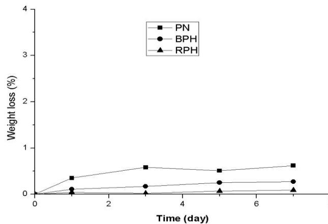
**Figure 9:** Weight loss of membrane in NaOH solution at pH=13.
