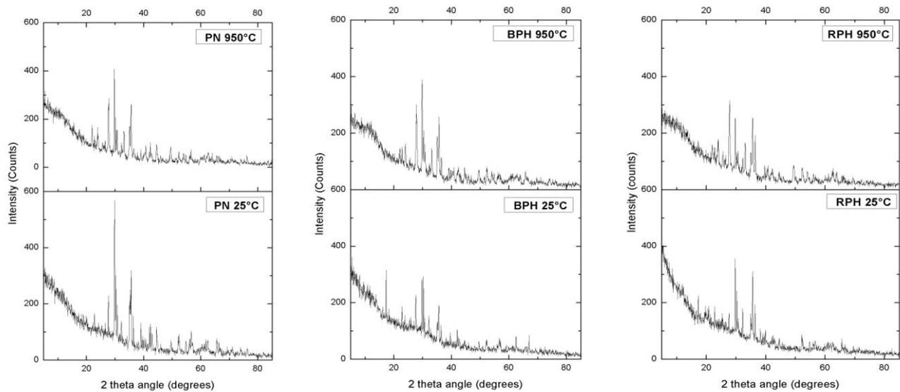
**Figure 3:** X-Ray diffractograms of natural and sintered pozzolans at 950 °C.
