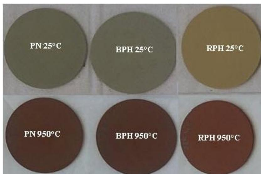
**Figure 7:** Views of elaborated membranes before and after sintering at 950 °C.
