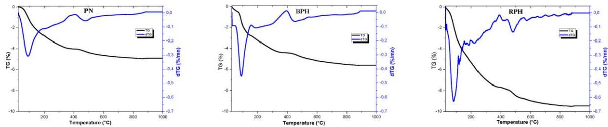
Figure 4: TGA and DTA of natural pozzolans.
