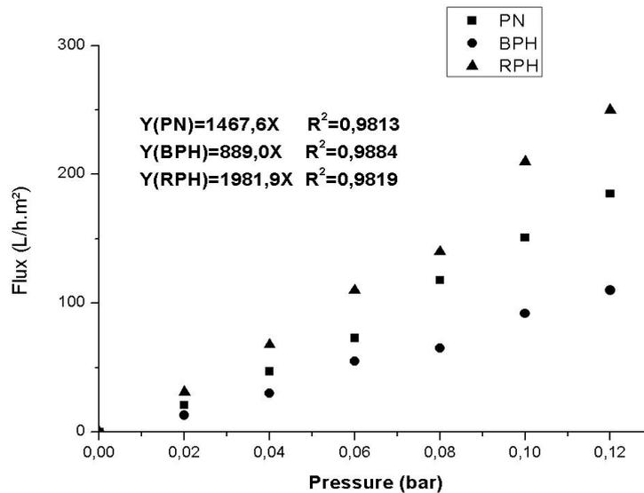
**Figure 10:** Variation of water flux as a function of transmembrane pressure.
