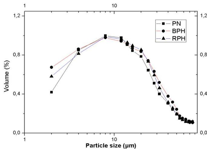
Figure 5: Particle size distribution of pozzolan powders.
