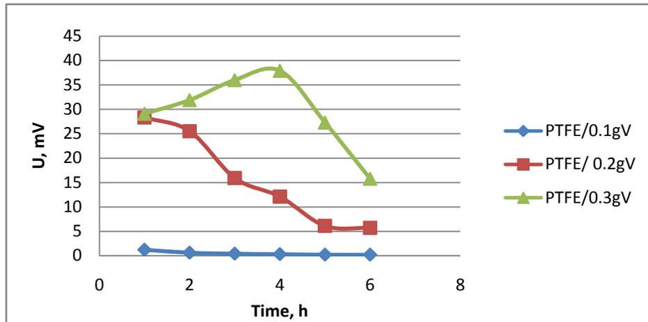
**Figure 10:** Voltages measured in the MFC with air cathodes modified with Polytetrafluoroethylene
