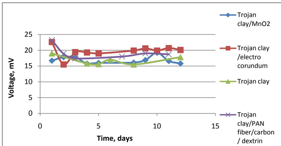
**Figure 9.** Voltages measured in the SMFC with ceramic membranes
