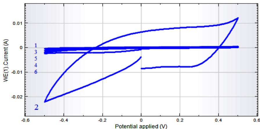
**Figure 11 :** Cyclic voltammetry of modified electrodes N1- reference electrode with Nafion; Cathode N2 - Nafion/Vulcan; Cathode N3 - Nafion/PANI; Cathode N4 - Nafion/ Polycarbazole; cathode N5 - Nafion/ Polynitrotosylcarbazole; cathode N6- Nafion/ ceramic powder.
