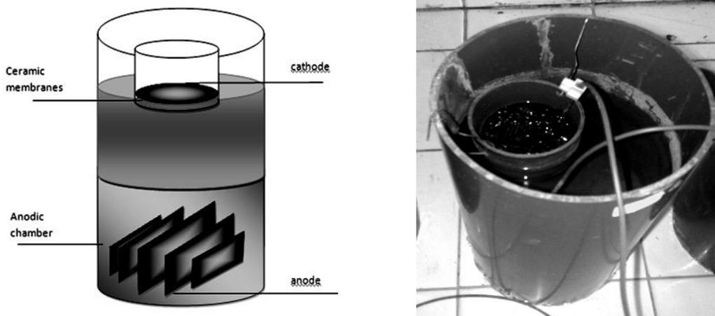
**Figure 3:** Design of the Sedimentation Microbial Fuel Cell (left) and real reactor (right) used in this study
