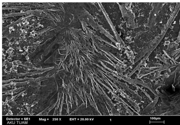
**Figure 2:** SEM images of PANI was chemically synthesized on stainless steel of SS304.
