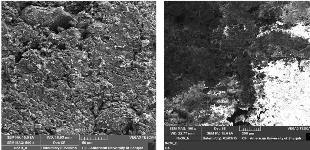
Figure 6: SEM of membranes Trojan clay and Trojan clay/PAN fiber/carbon/ dextrin
