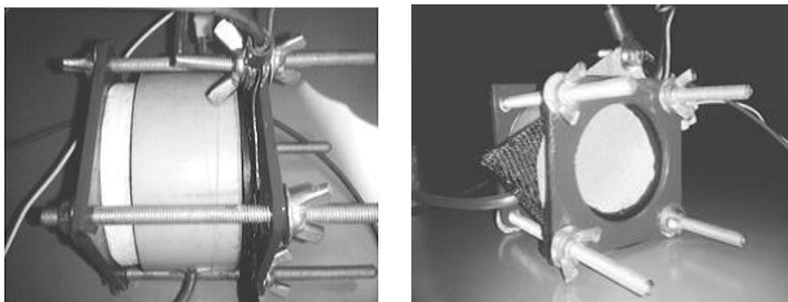
**Figure 4:** Real reactor of the Microbial Fuel Cell with air cathode used in this study
