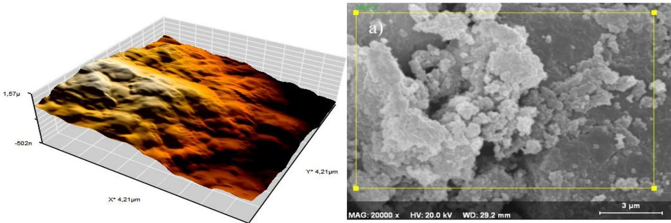
**Figure 1:** AFM images of PCz and SEM images of PCz was chemically synthesized on stainless steel of SS304.
