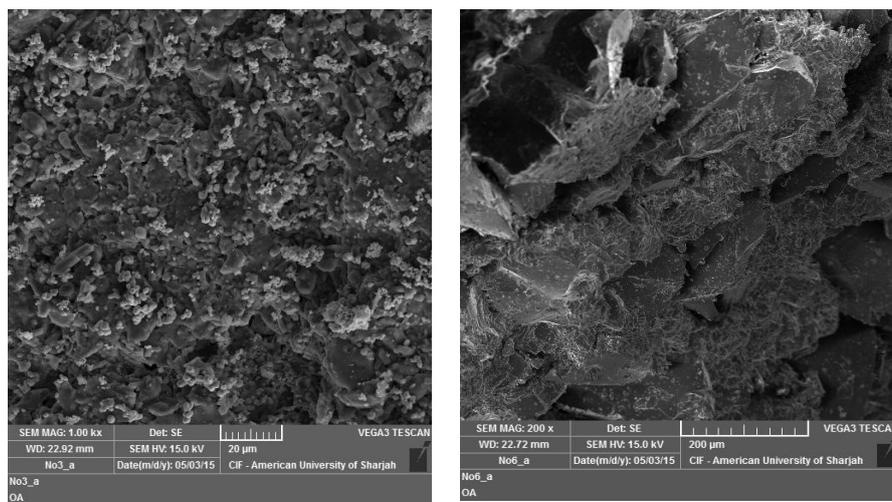
**Figure 5:** SEM of membranes Trojan clay/ $\text{MnO}_2$  and Trojan clay /electro corundum
