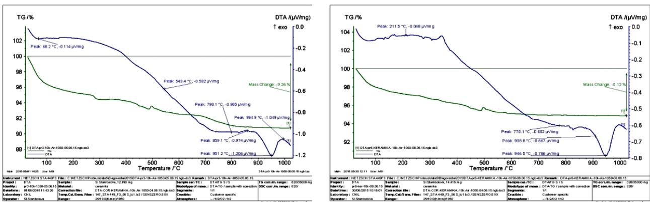
Figure 7: DTA and TG diagrams of membranes Trojan clay/MnO<sub>2</sub> and Trojan clay /electro corundum
