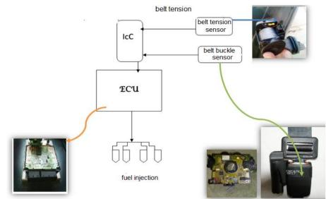
Figure 8: Smart seatbelt procedure
