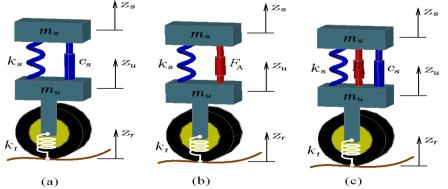
Figure 14:Quarter-car suspension systems: (a) Passive Suspension System, (b) Active Electromagnetic Suspension System and (c) Active Hydraulic Suspension System [18, 19]
