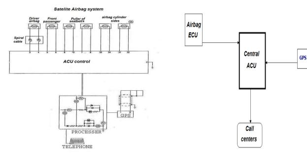
Figure 3:electrical circuit of smart air bag
