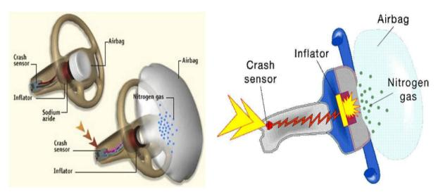
Figure 1: airbag structure and performance
