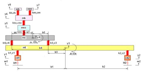
Figure 6: 10 dof vehicle vertical model
