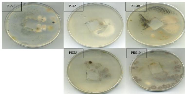
**Figure: 3** Macroscopic evolution of the different biopolymers after 45 days incubation at 30 °C in solid medium.
