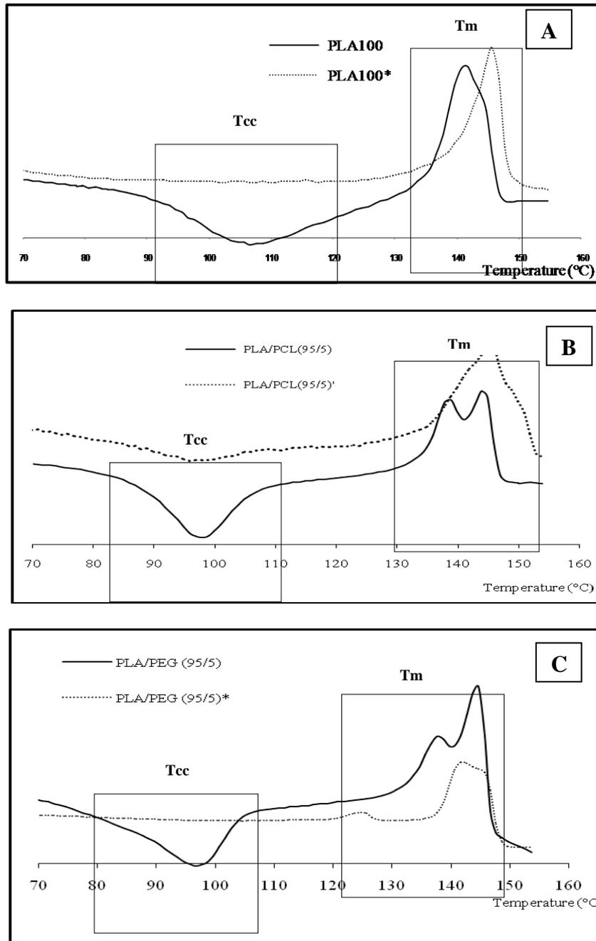
**Figure 4:** DSC thermograms of biopolymers before and after aerobic biodegradation. (A): PLA; (B): PCL5; (C): PEG5. \* : refers to samples after biodegradation. T<sub>m</sub>: melting temperature; T<sub>cc</sub>: cold crystallization temperature.
