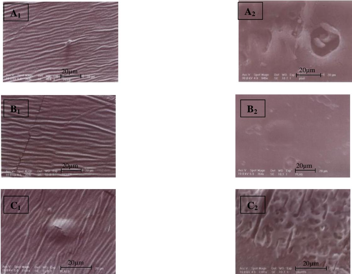
**Figure 5:** Morphologies of biopolymers observations by SEM before (A<sub>1</sub>): PLA; (B<sub>1</sub>): PCL5; (C<sub>1</sub>): PEG5 and after (A<sub>2</sub>): PLA; (B<sub>2</sub>): PCL5; (C<sub>2</sub>): PEG5 aerobic biodegradation.
