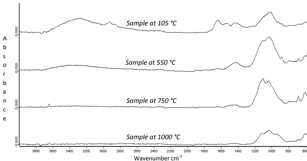
**Figure 5:** ATR-FTIR spectra obtained for sludge 2 treated at different temperatures.
