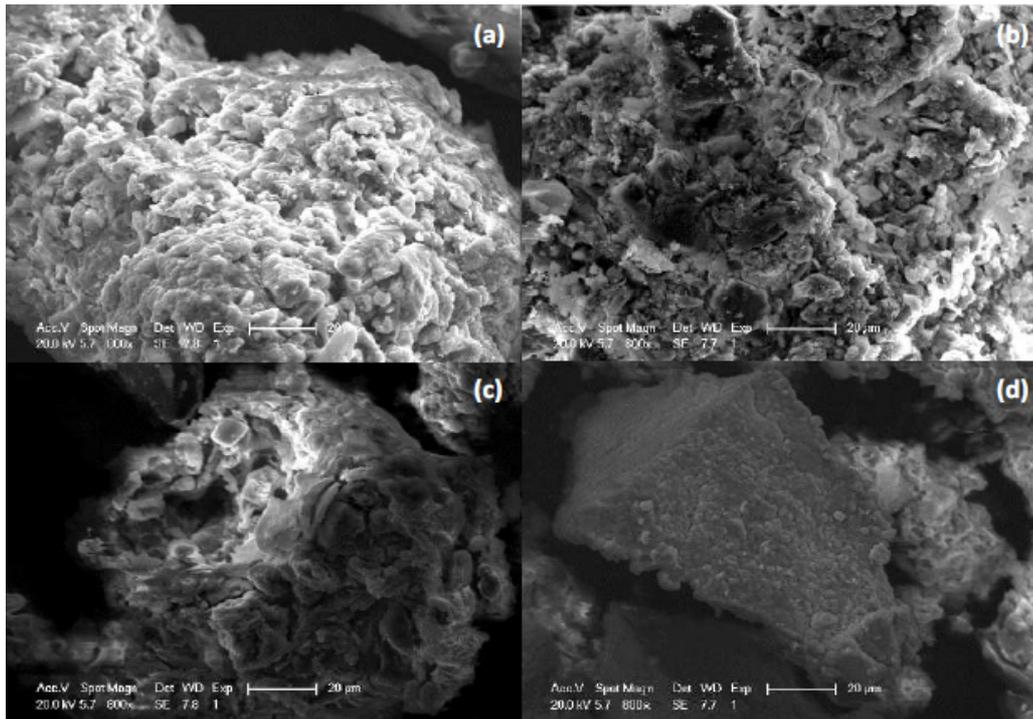
**Figure 4:** SEM photography of sludge 2 treated at (a) 105°C, (b) 550°C, (c) 750°C and (d) 1000°C.
