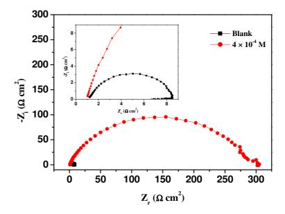
**Figure 5:** Nyquist plot of mild steel in the absence and presence of MPD in 1M sulphuric acid solution.
