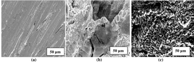
**Figure 8:** Scanning electron micrographs of mild steel surface of (a) polished mild steel (b) mild steel in 1M  $H_2SO_4$  (c) inhibited mild steel in 1M  $H_2SO_4 + 4 \times 10^{-4} M$  MPD.
