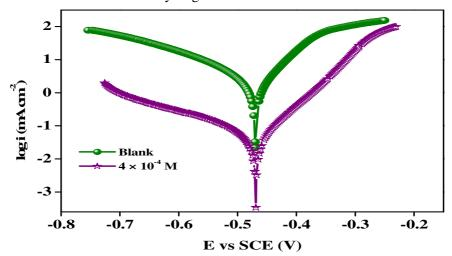
Figure 4: Tafel polarization curve in absence and presence of MPD on mild steel surface in 1M sulphuric acid
