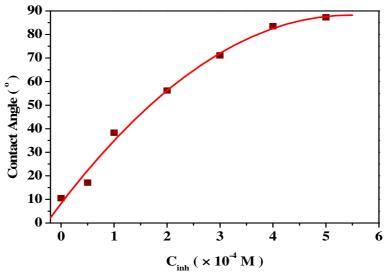
Figure 7: Variation of contact angle of mild steel surface to the acid solution with inhibitor concentration
