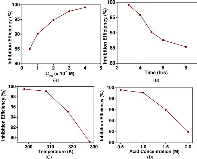
**Figure2:** Variation in inhibition efficiency in 1 M sulphuric acid on mild steel of surface area 20 cm<sup>2</sup> with (A) different concentration of MPD (B) different immersion time (C) different temperature and (D) different acid concentration range; using weight loss data.
