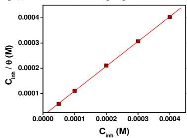
Figure 3. Langmuir's Adsorption isotherm plot for the adsorption of MPD in sulphuric acid on the surface of mild steel.
