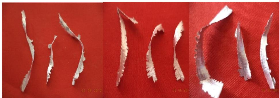
**Figure 9:** Chip formed in Graphite reinforced composite at 3000 rpm, 50 mm/min and 6mm
