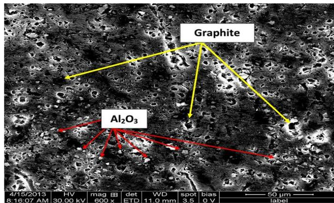
**Figure 3:** SEM image of AA 6063-6wt-% Al<sub>2</sub>O<sub>3</sub>-1wt-% Gr
