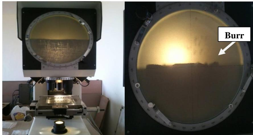
**Figure 2:** SP-300 SIPCON profile projector and burr height
