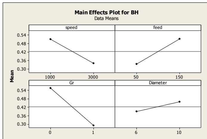
Figure 4: Main effects plot for Burr Height
