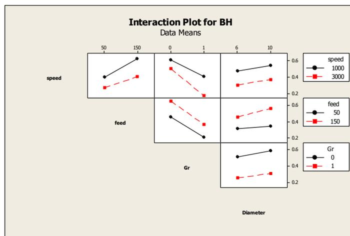
Figure 5: Interaction plot for Burr Height
