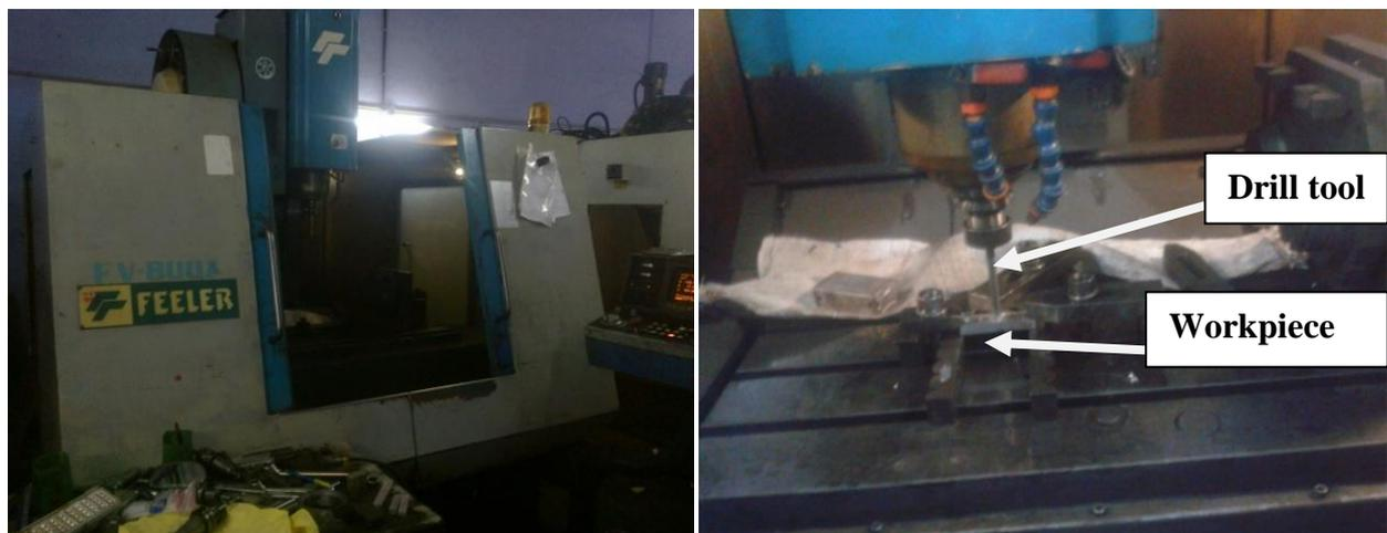
**Figure 1:** Vertical machining centre and drilling setup
