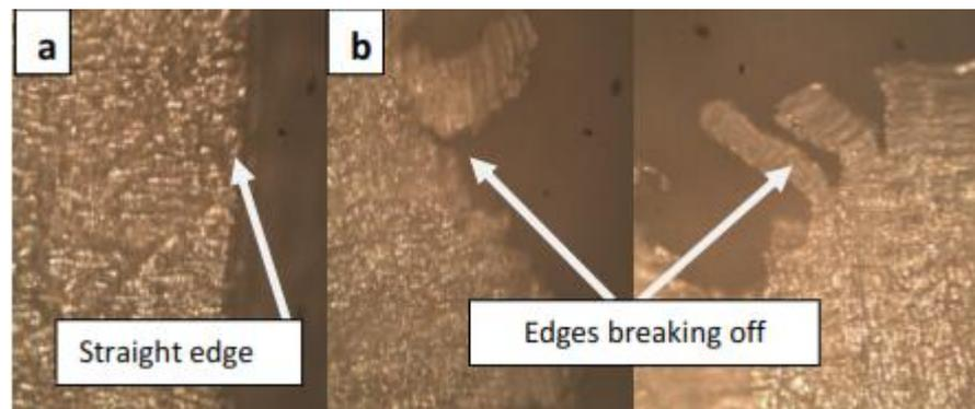
**Figure 10:** Chip edges formed in (a) Non-Graphite composite (b) Graphite reinforced composite
