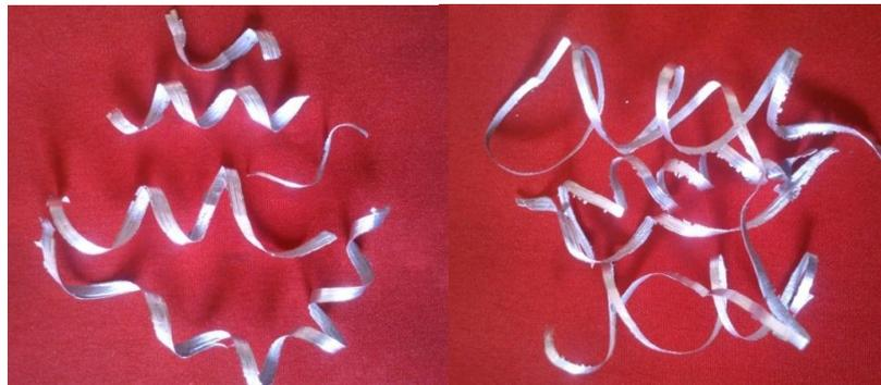
**Figure 8:** Chip formed in Non-Graphite composite at 3000 rpm, 50 mm/min and 6mm
