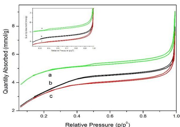
**Fig 2** Adsorption-desorption isotherms of nitrogen of TiO<sub>2</sub>OH-IBU with different water ratio, a) 1:8:8 b) 1:16:8 c) 1:24:8
