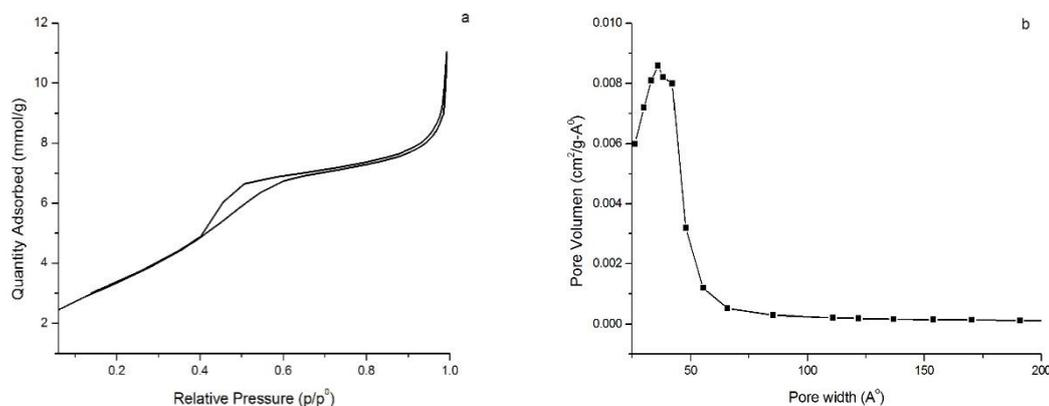
**Fig 3** a) Adsorption-desorption isotherms of nitrogen b) BJH Pore diameter distribution of TiO<sub>2</sub>OH Ref (1:24:8)
