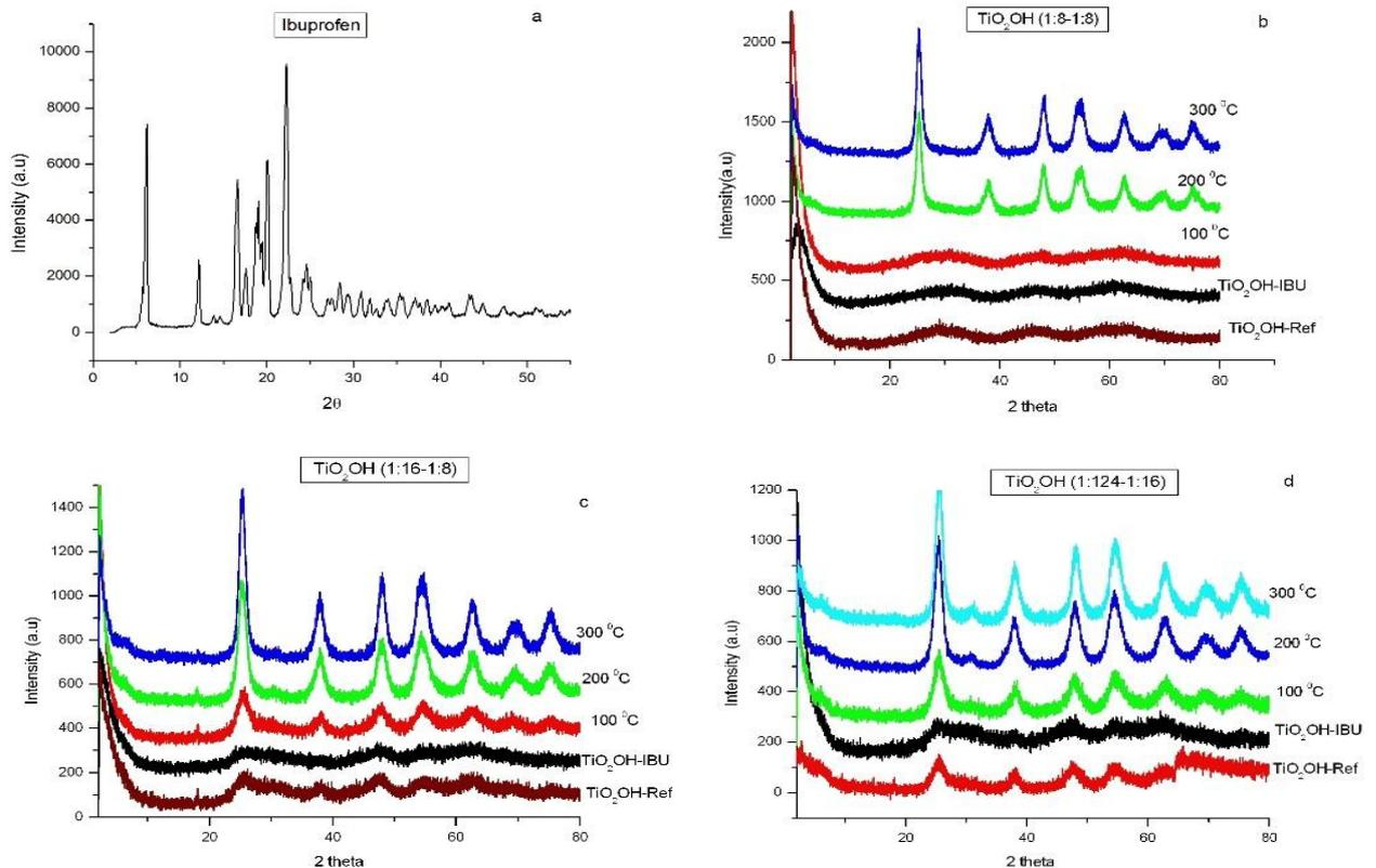
**Fig. 7.** Diffraction patterns (XRD) a) pure Ibuprofen, b)TiO<sub>2</sub>OH-Ref and TiO<sub>2</sub>OH-IBUcompositesat various temperatures
