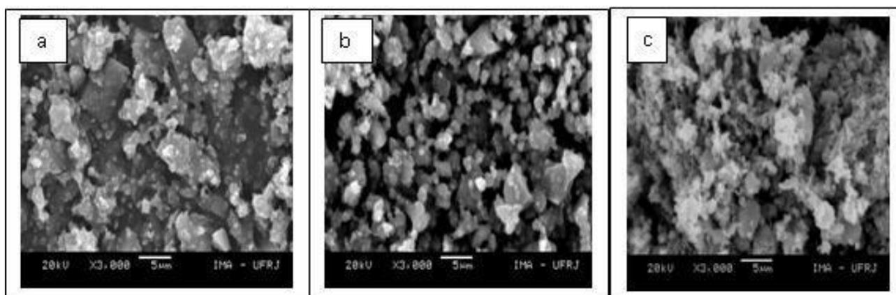
Fig 6 Scanning electron micrographs (SEM) of TiO<sub>2</sub>OH-Ibuprofen, a) 1:8 b) 1:16, c) 1:24.
