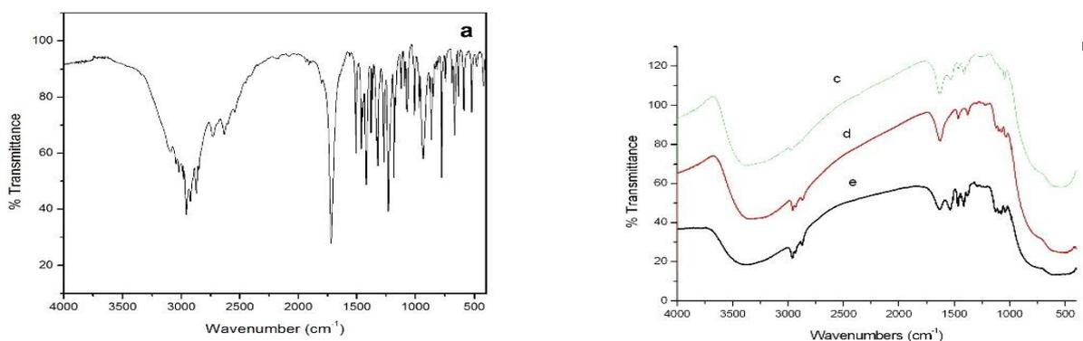
**Fig 4** Fourier transforms infrared spectroscopy (FTIR) spectra of a) Ibuprofen (IBU), b) TiO<sub>2</sub>OH-Ibuprofen with different water ratios c) 1:24:8 d) 1:16:8 e) 1:8:8
