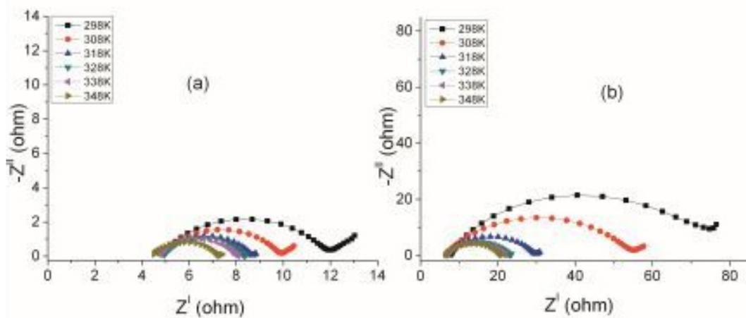
**Figure 2:** Nyquist plots of the GPEs at different temperatures (a) S2 and (b) A2.
