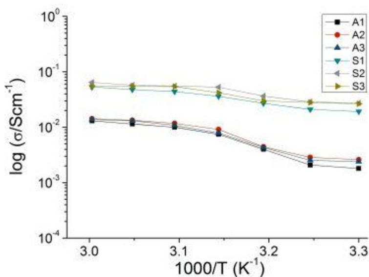
**Figure 1:** Variations of bulk conductivities of GPEs with different temperatures.
