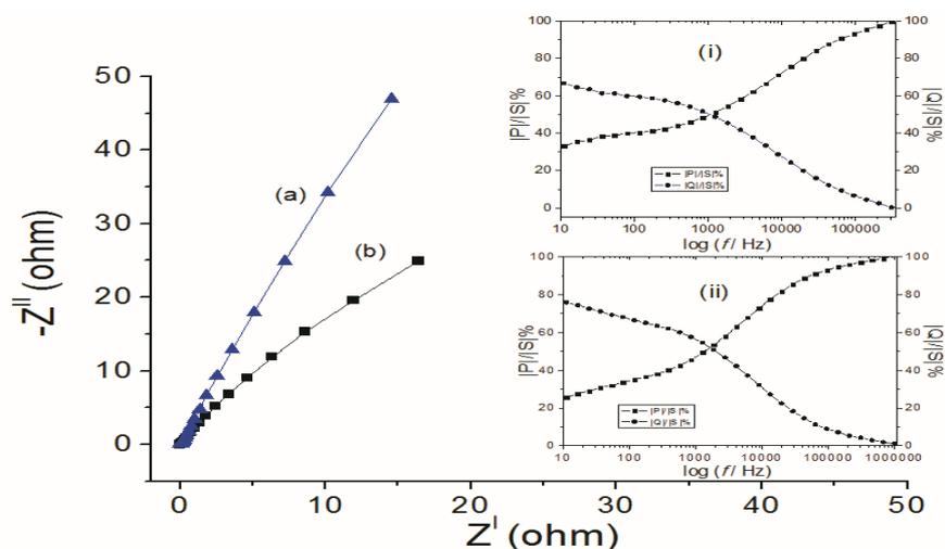
**Figure 10:** AC impedance plots of (a) A2 and (b) S2 supercapacitors [inset: Plots of normalized reactive power  $QI/|S|\%$  and active power  $PI/|S|\%$  versus frequency (Hz) of (i) A2 and (ii) S2].
