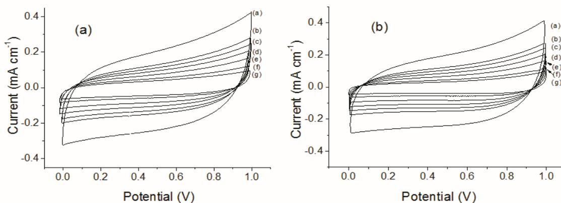
**Figure 9a and b:** CVs of EDLC containing A2 and S2 supercapacitors, respectively at (a)  $50 \text{ mV s}^{-1}$ , (b)  $25 \text{ mV s}^{-1}$ , (c)  $20 \text{ mV s}^{-1}$ , (d)  $15 \text{ mV s}^{-1}$  (e)  $10 \text{ mV s}^{-1}$ , (f)  $5 \text{ mV s}^{-1}$ , and (g)  $2 \text{ mV s}^{-1}$
