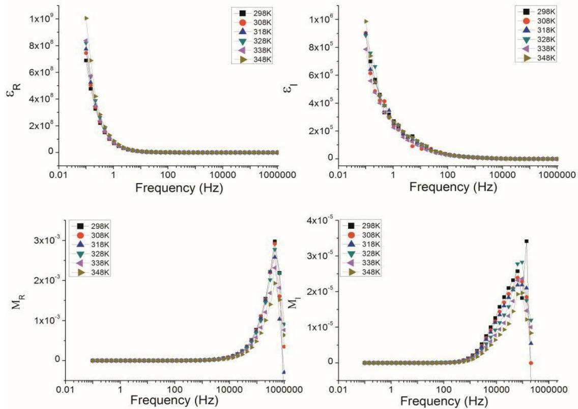
**Figure 3.** Plots of dielectric studies versus frequency at different temperatures (a) dielectric constant, (b) dielectric loss, (c) real part of electric modulus, and (d) imaginary part of electric modulus of A2.
