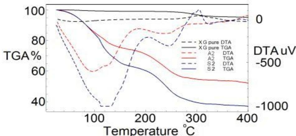
Figure 6: TGA and DTA measurements of pure XG, S2 and A2.
