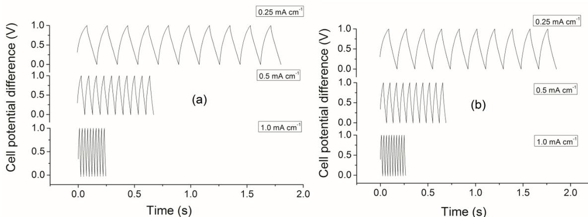
**Figure 11a and b:** Galvanostatic charge/discharge plots for A2 and S2 supercapacitors at different current densities, respectively.
