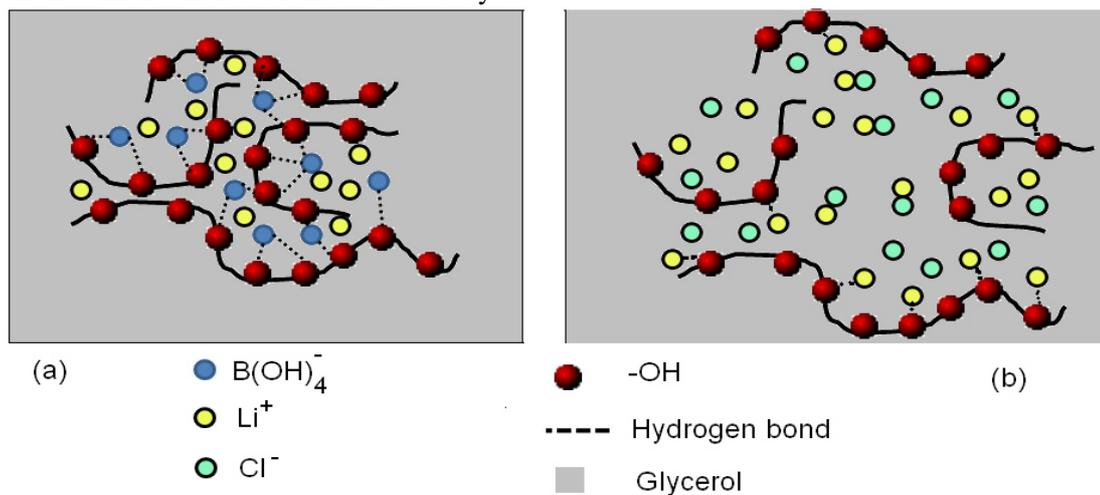
**Figure 8:** Predicated mechanism of ionic conduction in GPEs (a)  $\text{Li}_2\text{B}_4\text{O}_7$  doped GPE and (b)  $\text{LiClO}_4$  doped GPE
