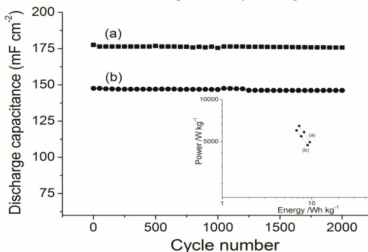
**Figure 12:** Discharge capacitance versus number of cycles and Ragone plot (inset) of (a) S2 and (b) A2. (Current density:  $1 \text{ mA cm}^{-2}$ )
