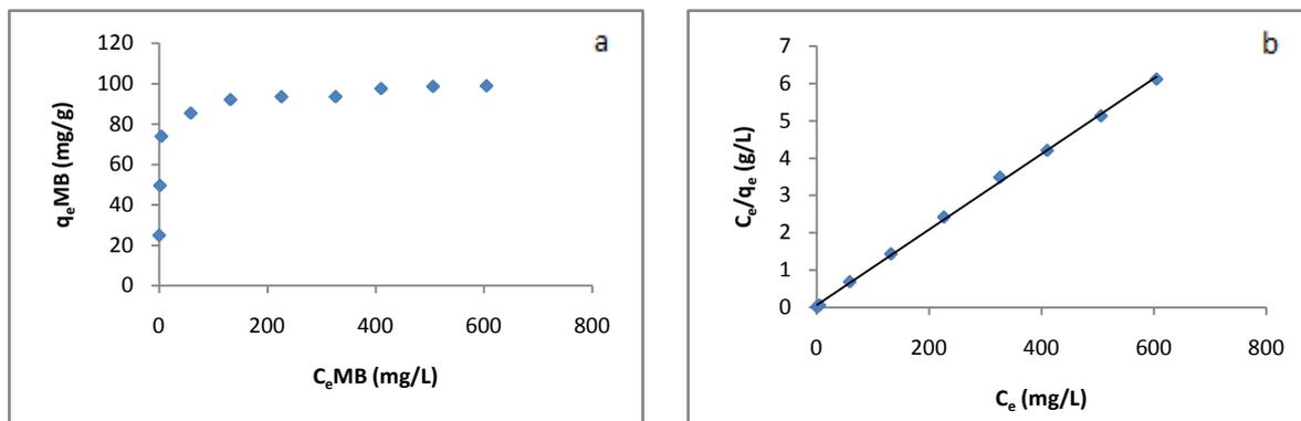
**Figure 1:** (a) Biosorption isotherm and (b) linear plot of Langmuir isotherm for the biosorption of methylene blue on the biosorbent (biosorbent dose 4 g/L, MB initial concentrations: [100-1000 mg/L],  $t = 24$  h, temperature:  $25^\circ\text{C}$ ).
