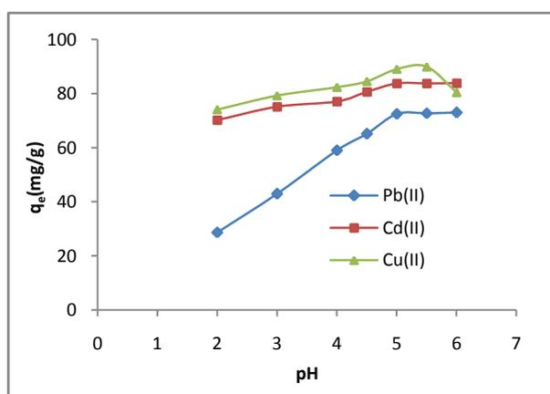
**Figure 3:** Effect of pH on the biosorption of metal ions by the biosorbent at temperature = 25°C, contact time = 120min, metal ions initial concentration = 50mg/L, biosorbent dose = 0,5g/L and agitation speed = 250rpm.
