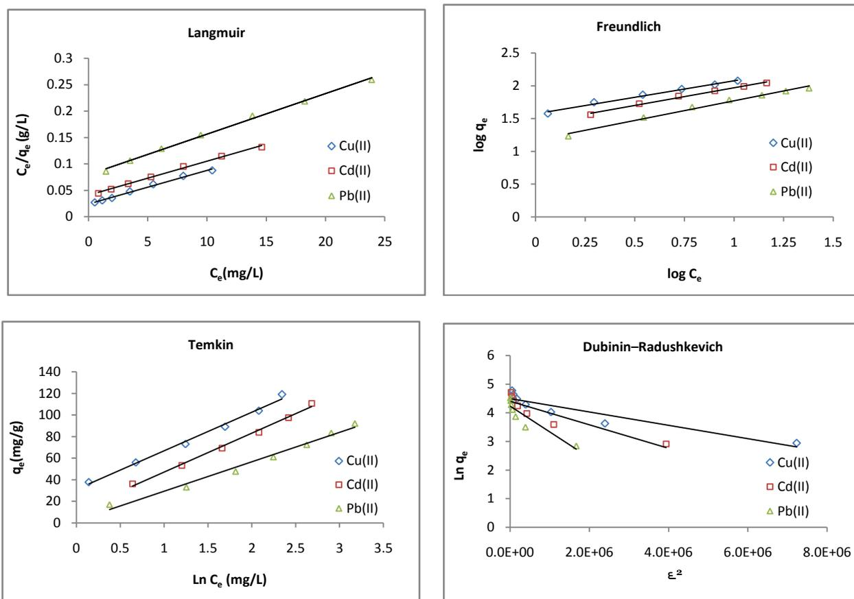
**Figure 6:** Biosorption isotherms of Cu(II), Cd(II) and Pb(II) onto the biosorbent at temperature = 25°C, biosorbent dose = 0.5g/L, initial concentrations = [10-70mg/L], contact time = 120min, pH = 5 and agitation speed = 250rpm.
