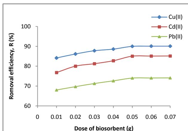
**Figure 4:** Effect of biosorbent dose on the biosorption of metal ions by the biosorbent at temperature = 25°C, contact time = 120min, metal ions initial concentration = 50mg/L, pH = 5 and agitation speed = 250rpm.
