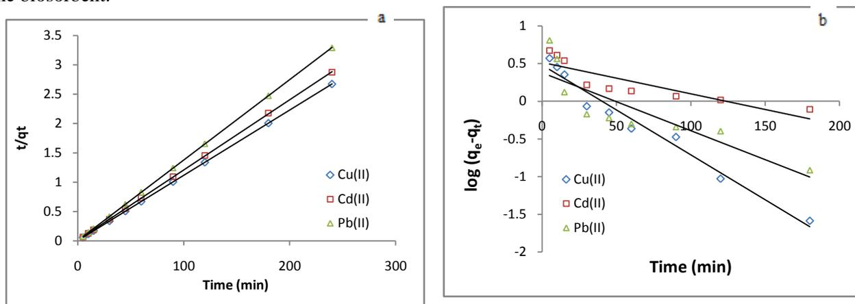
**Figure 7:** (a) Pseudo-second-order and (b) Pseudo-first-order kinetics plots for the removal of Cu(II), Cd(II) and Pb(II) by the biosorbent.
