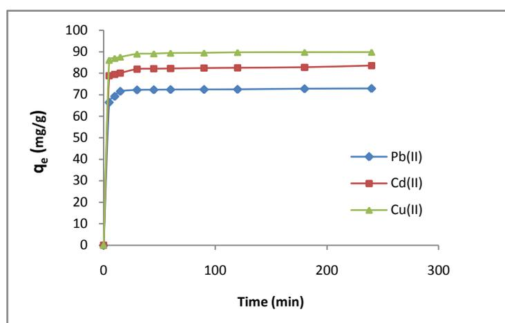
**Figure 5:** Effect of contact time on the biosorption of metal ions by the biosorbent at temperature = 25°C, biosorbent dose = 0.5g/L, metal ions initial concentration = 50mg/L, pH = 5 and agitation speed = 250rpm.
