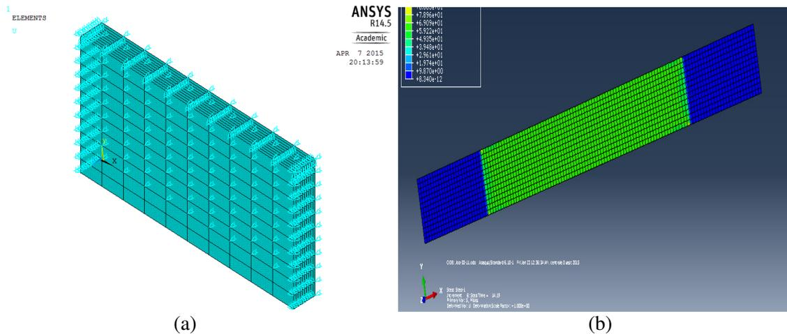
**Figure 10:**(a) The meshed structure with SOLID45 element, (b)Traction simulation results by abaqus.
