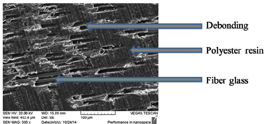
**Figure 9 :** SEM micrograph of a sample aged during 90 days at 80 °C
