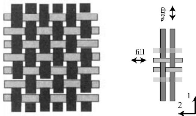
**Figure 1:** Schematic representation of woven fabric architecture [17]
