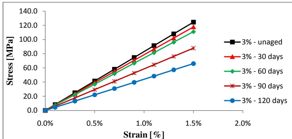
**Figure 6 :** Experimental curve of the tensile test for polyester fiber glass composites with 3% of catalyst.
