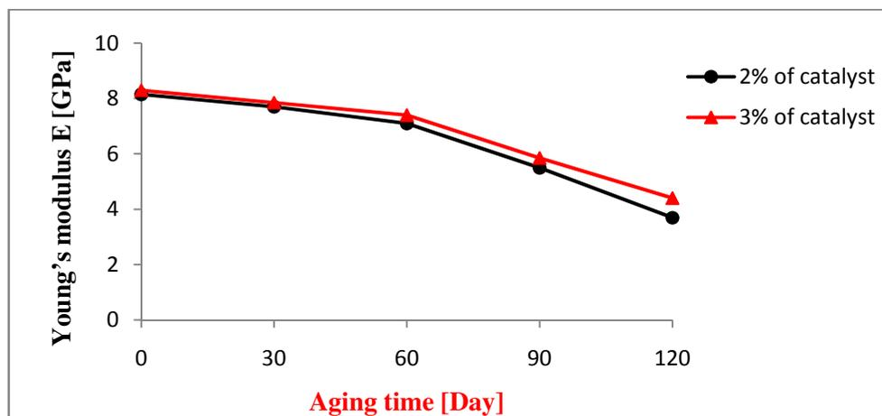
**Figure 7:** Young's modulus variation according to aging time at  $80^\circ\text{C}$  for polyester fiberglass composites with 2% of catalyst and 3% of catalyst.
