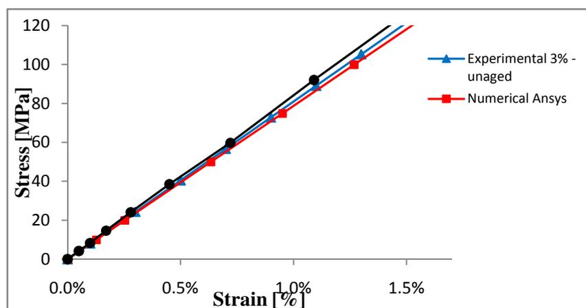
**Figure 11 :** numerical and experimental comparison for unaged samples with 3% of catalyst
