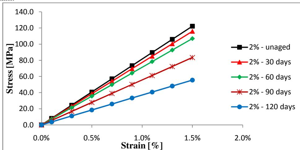
Figure 5: Experimental curve of the tensile test for polyester fiber glass composites with 2% of catalyst.
