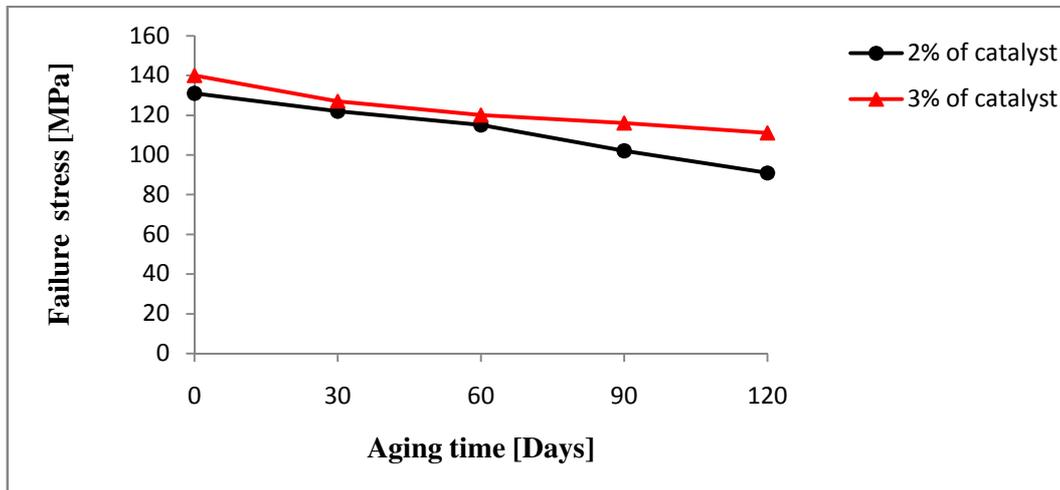
**Figure 8 :** Failure stress variation according to to aging time at 80 °C for polyester fiber glass composites with 2% of catalyst and 3% of catalyst.
