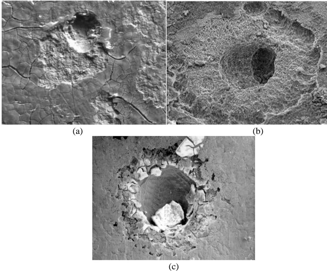
Figure 1 (a) Pit formation, (b) Growth of pit and (c) Pitted steel
