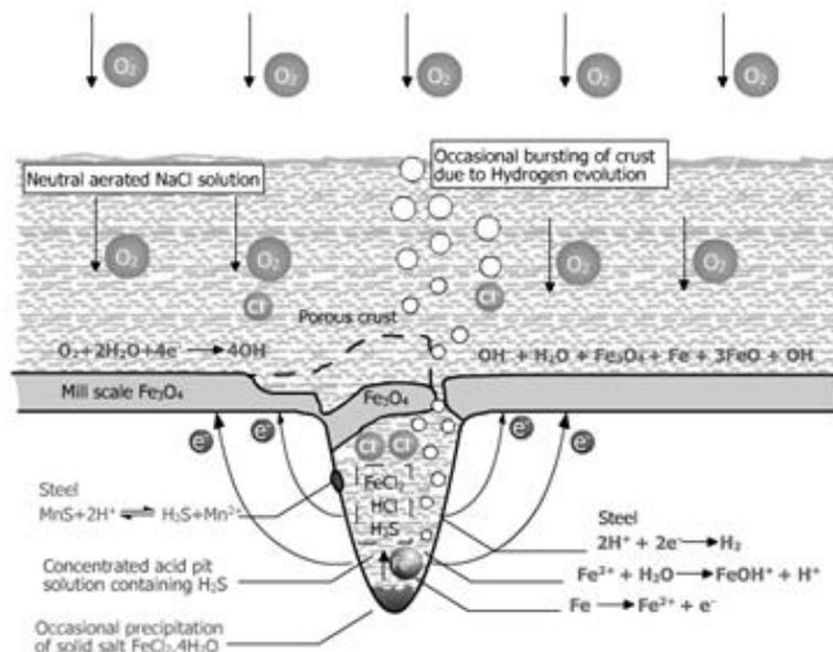
Figure 2 Electrochemical reactions that occur when a pit is initiated at sulphide inclusions in a carbon steel [16].
