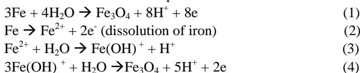
In the presence of  $\text{Cl}^-$ , the hydrolysis of  $\text{Fe}^{2+}$  is accelerated, as shown in the reactions below;
