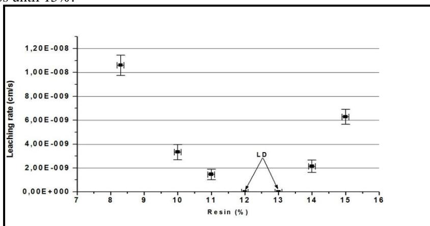
Figure 8: leaching rate variation activity relative to the percentage of the resin incorporated by formulations. LD : the value of detected activity is below the detection limit of the detector. LD= 0.27 Bq/Kg.
