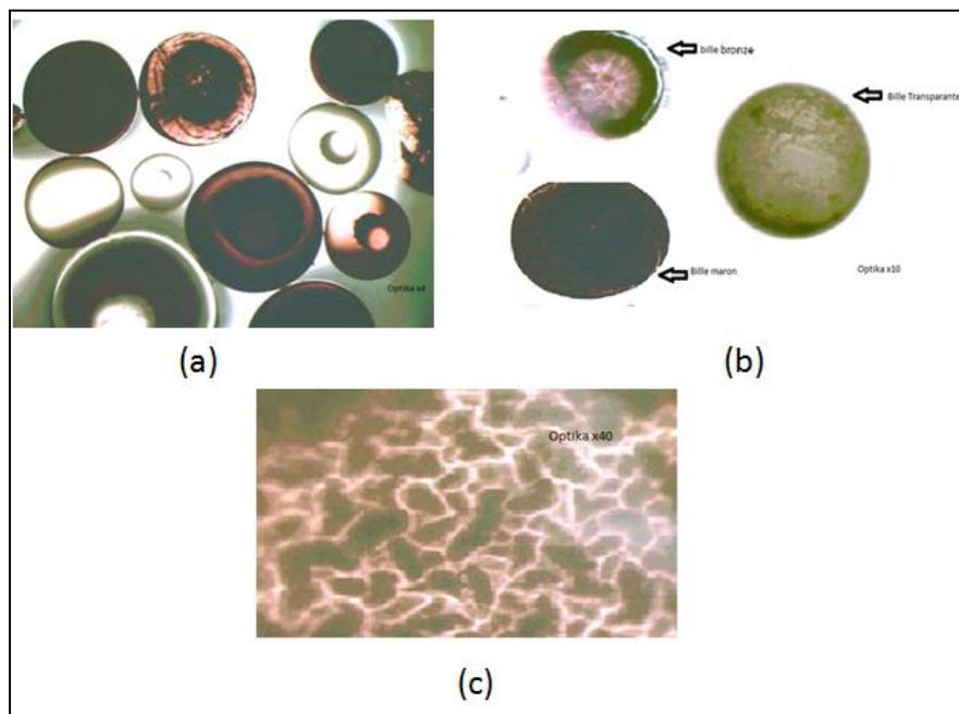
**Figure 2:** resin beans observed with different enlargement: (a): an enlargement of 4; (b): an enlargement of 10; (c): an enlargement of 40.
