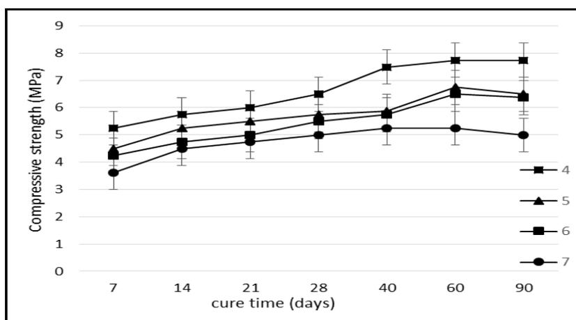
**Figure 4:** strength behavior for formulations 4, 5, 6, 7 at different curing time.
