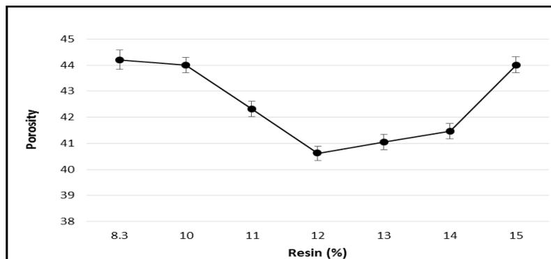
Figure 6: The variation of porosity relative to the percentage of the resin incorporated by formulations.
