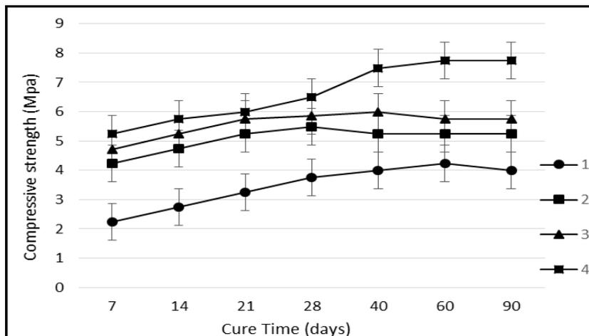
**Figure 3:** strength of the package of formulations 1, 2, 3, 4 at different curing time.
