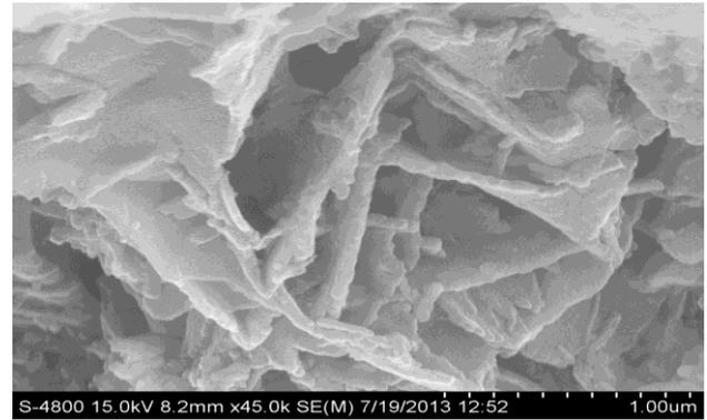
**Fig-2(b).** SEM images of adsorption of acid violet 19 dye on PANI-Fe<sub>2</sub>O<sub>3</sub> nano-composites.
