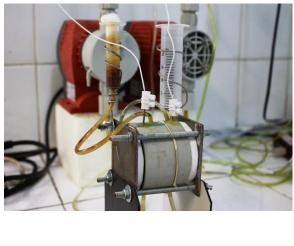
Fig. 1. Design of the Microbial Fuel Cell (left) and real reactor (right) used in this study
