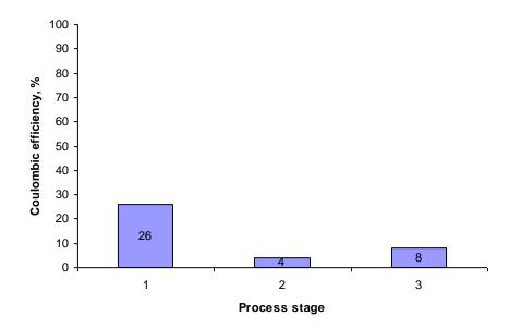
**Fig. 3.** Coulombic efficiency of the MFC during the different stages of the process  $(1^{st} \text{ stage} - 0 - 48h; 2^{nd} \text{ stage } 48-168h; 3^{rd} \text{ stage } 168-196h)$
