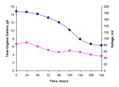
Fig. 2. Total Organic Carbon (•) and Voltage (•) vs. Time observed in the experiments with MFC
