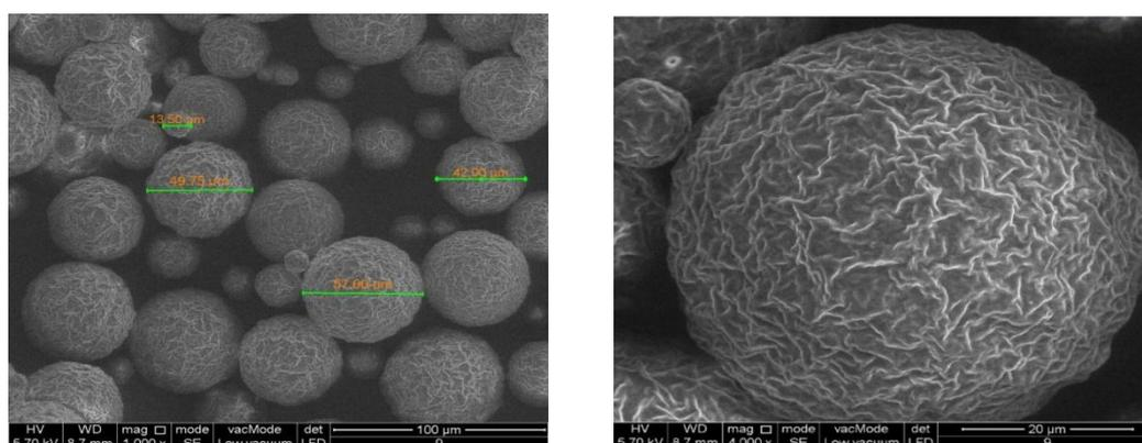
**Figure 4:** SEM of spherical microspheres; TA4.
