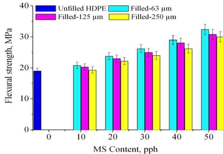
Figure 5: Flexural strength graph for MS/HDPE composites
