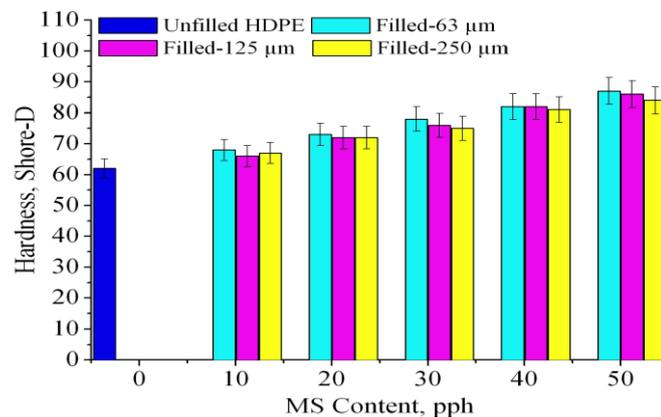
Figure 7: Hardness graph for MS/HDPE composites
