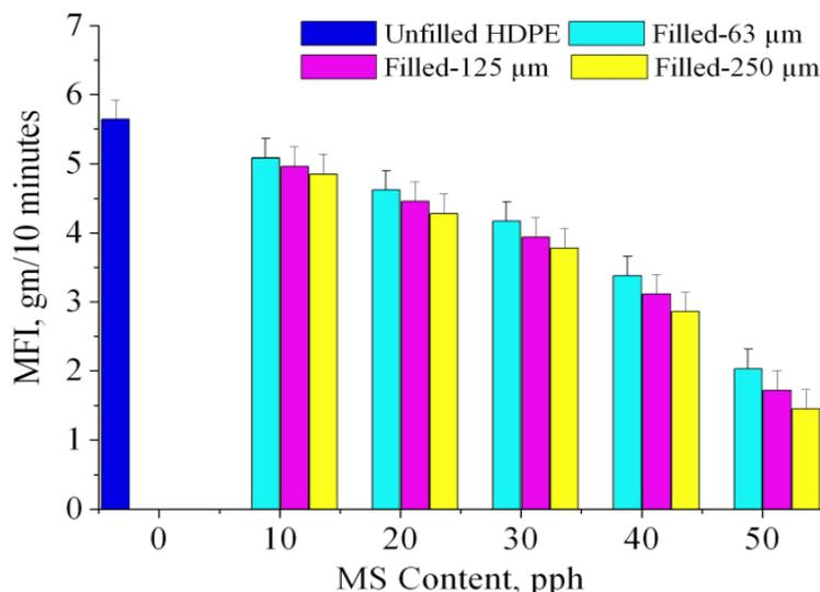
Figure 1: Melt Flow Index graph for MS/HDPE composites
