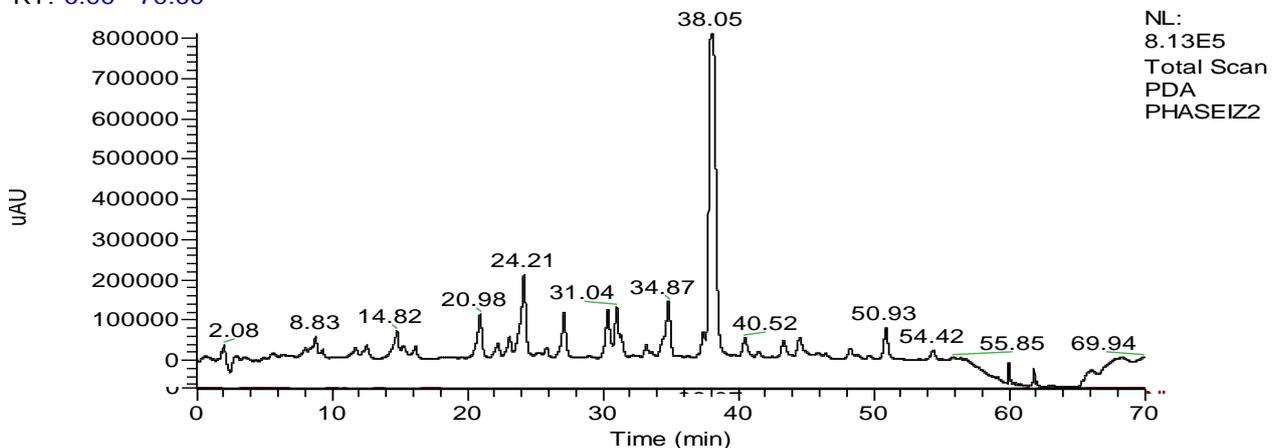
Figure 6: LC Chromatogram of diethyl ether fraction (DEF) obtained from olive leaves.
