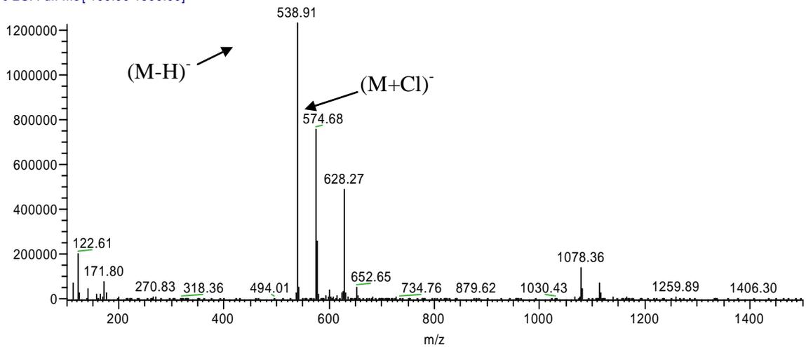
**Figure 2:** Mass spectra of oleuropein standard in negative mode eluted at 33.25 min.
