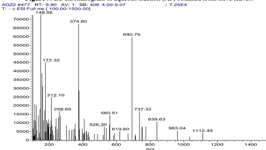
Figure 10: Mass spectra of oleuropein pentose found in aqueous fraction (AF) in negative mode.
