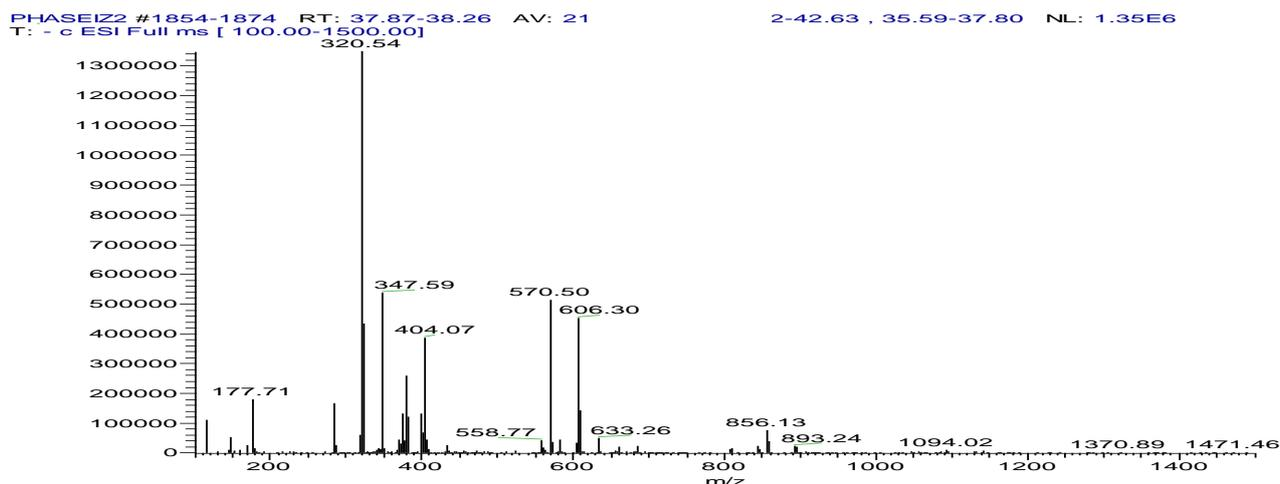
**Figure 7:** Mass spectra of ligstroside acid found in diethyl ether fraction (DEF) in negative mode.
