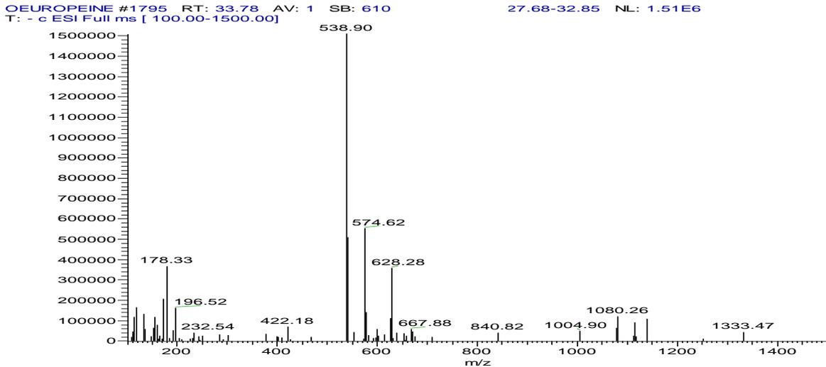
Figure 4: Mass spectra of oleuropein standard in negative mode eluted at 33.78 min.
