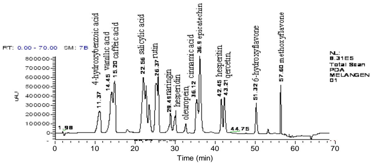
**Figure 1:** LC Chromatogram of the phenolic standards (4-hydroxybenzoic acid, vanillic acid, caffeic acid, salicylic acid, rutin, hesperidin naringin, oleuropein, cinnamic acid, epicatechin, hesperitin, quercetin, 6-hydroxyflavone and methoxyflavone)
